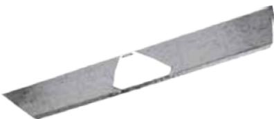
Designed to be installed with the One-Shot ceiling speakers, these pans support the ceiling tile to minimise sag and reduce damage to soft tiles. Fits inside the "T-bars" for maximum support for the tile. Recommended for use with mineral fibre and acoustic ceiling tiles.
