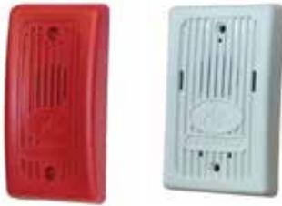
The GX93 is ideal for applications where a dependable alarm signal is required in hotels, dormitories, apartments, and other installations. The unit is shipped with J1 inserted for an ISO8201 T3 tone pattern. Remove J1 for continuous horn signal. The GX93 is intended for indoor installation only. This appliance is not weather-proofed for outdoor applications.
