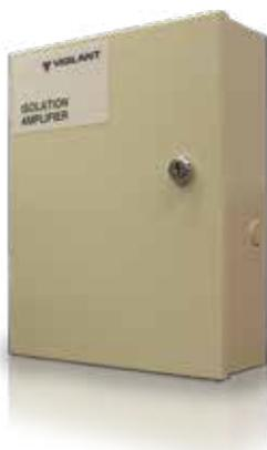
The FP1135 Isolation Amplifier connects to an existing 100V speaker line and reproduces this signal at up to 60W load on a separate supervised 100V line. It is suitable for use with speech, music and warning tones. The 100V output line from the amplifier is electrically isolated from the input 100V line, thus separating noise or other signals on the input line from the output. The Isolation Amplifier requires a nominal supply of 27Vdc.
