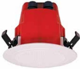
The 'One-Shot' PA speaker and grille is designed to install easily into 10 to 13mm gyprock/plaster/acoustic ceilings. Simply drill the required size hole, terminate the wiring and push the speaker into the ceiling until it snaps into place. They are designed to meet the requirements of AS ISO7240.24, with a cover and 22µF capacitor. The transformer has 5 power taps from 0.33 to 5W and a 4 way wire-protected terminal block.
