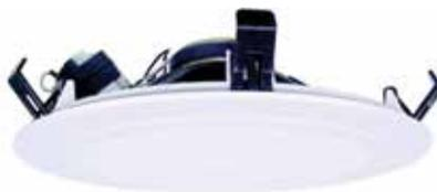
The 'One Shot' PA speaker and grille is designed to install easily into 10 to 13mm gyprock/plaster/acoustic ceilings. Simply drill the required size hole, terminate the wiring and push the speaker into the ceiling until it snaps into place. They are designed to meet the requirements of AS2220.1, with a transformer cover (not shown in the image) and 22µF capacitor. The transformer has 5 power taps from 0.33 to 5W and a 4 way terminal block.
