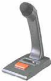
The SU0169 Paging microphone is a desktop dynamic microphone with a cardioid polar pattern. It features a short-off press to talk switch with an open-off type extra switch. It has low handling noise and a 600 ohm balanced output impedance. The SU0169 is finished in a grey ABS body with a zinc plated wire mesh head. Compatible with FP0539 and FP0902 Paging Consoles.
