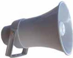
The EA0013 ABS horn speaker has a screwdriver adjustable power tap switch and a 22µF bipolar isolation capacitor to permit line monitoring. A 4 core loop through flying lead is provided.
