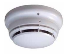
TrueAlarm photoelectric smoke detectors use a stable pulsed LED light source and a silicon photodiode receiver to provide consistent and accurate low power smoke sensing. Seven CIE. selected sensitivity levels are available for each detector. Used in conjunction with the Simplex 4100ES/4100U series of CIE, the 4098-9714EA has a high degree of nuisance alarm immunity thanks to advanced algorithms.
