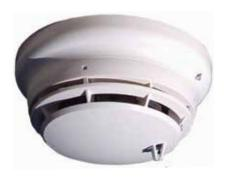
This multi-sensor detector combines the TrueAlarm photoelectric smoke sensor with a fast-acting, accurate TrueAlarm thermal sensor in a single detector/base assembly. Each multi-sensor's smoke and heat sensing element provides data for evaluation at the CIE where four independent detection modes are evaluated:
