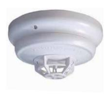
TrueAlarm heat detectors provide rate-compensated, fixed temperature sensing, selectable with or without rate-of-rise temperature sensing. Due to its small thermal mass, the detector accurately and quickly measures the local temperature for analysis at the CIE. Rateof-rise temperature detection is selectable at the CIE. Fixed temperature sensing is independent of rate-of-rise sensing. Configurable for either Type A or Type B as per AS 1603.1.
