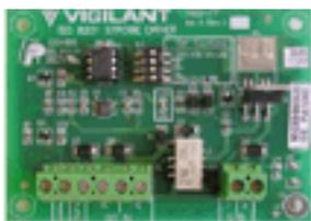
The ISO 8201 Strobe Driver generates an ISO 8201 compliant "T3" pattern for the Multi-Candela strobe 4906-9104. It connects directly to a supervised relay output of a fire alarm panel and drives one or more lines to strobes with a synchronised T3 pattern. The fire alarm panel's output supervision supervises the wiring from the panel to the strobes. The output signals of up to 5 modules can be synchronised.
