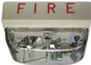
The 4906-9104 Multi-Candela strobe is a high output xenon strobe capable of signalling evacuation using the ISO 8201 "T3" temporal pattern, as required by AS1670.4-2004 and AS 1670.1-2004. It is ceiling mounted and produces white light with a link-selectable intensity of 15cd, 30cd, 75cd or 110cd. It is usually controlled by the ISO 8201 Strobe Driver Module (PA1043) or a QE90 STRM Strobe Relay Module. A 24V output cannot be used.
