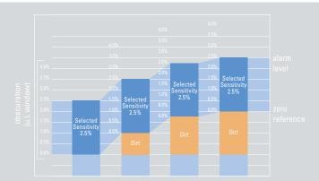
*MX* sensors are engineered to maintain their present levels of sensitivity. As dirt accumulates, the sensors self-adjust, notifying operators of Almost Dirty, Dirty and Excessively Dirty conditions long before they trigger a nuisance alarm. This lets you schedule maintenance on both Dirty and Almost-Dirty sensors at the same time, minimising your facility costs.
