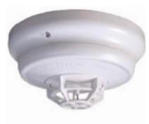
TrueAlarm heat detectors provide rate compensated, fixed temperature sensing, selectable with or without rate-of-rise temperature sensing. Due to its small thermal mass, the detector accurately and quickly measures the local temperature for analysis at the c.i.e. Rate-of-rise temperature detection is selectable at the c.i.e. Fixed temperature sensing is independent of rate-of-rise sensing. Configurable for either Type A or Type B as per AS 1603.1.
