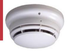
TrueAlarm photoelectric smoke detectors use a stable pulsed LED light source and a silicon photodiode receiver to provide consistent and accurate low power smoke sensing. Seven c.i.e. selected sensitivity levels are available for each detector. Used in conjunction with the Simplex 4100/4100U series of c.i.e., the 9714EA has a high degree of false alarm immunity thanks to advanced algorithms. The TrueAlarm detectors are mounted on to the 4098-9789EA addressable base or 4098-9794EA sounder base.
