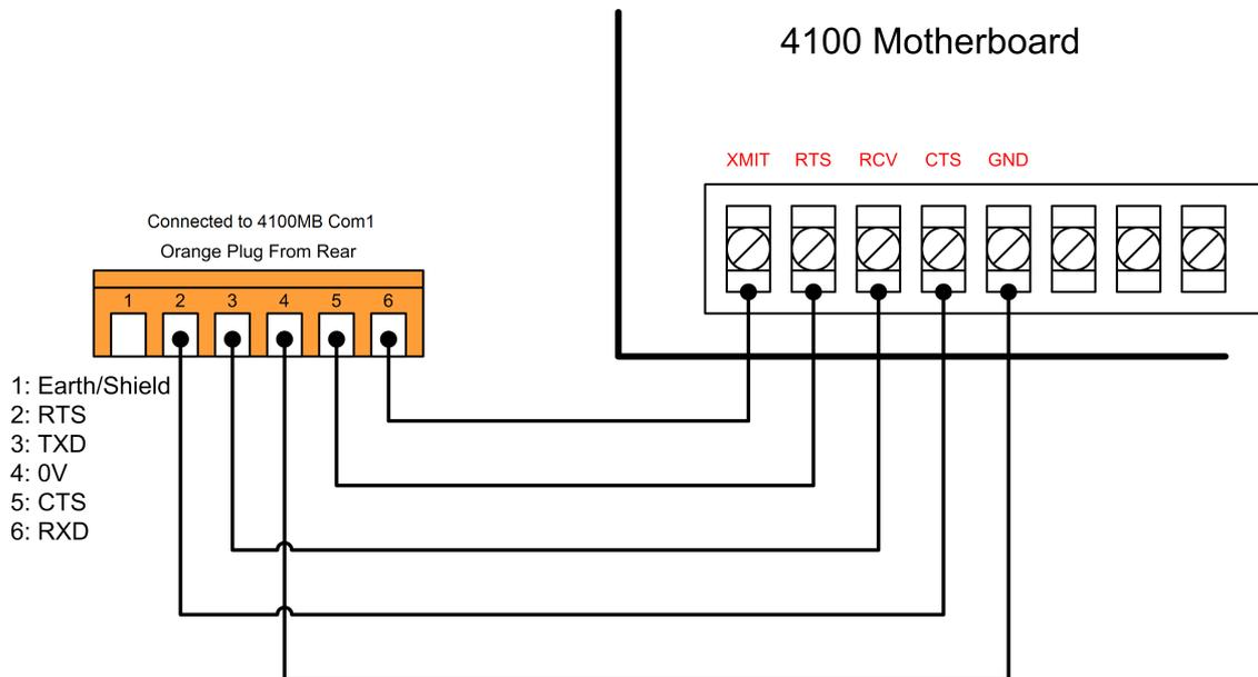
Figure 5: Connection of 4100MB to Terminals on 4100 Motherboard.
