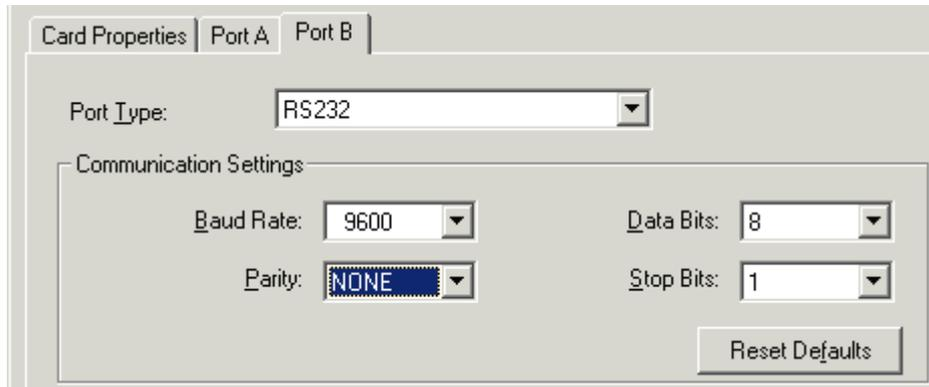
Figure 8. Port Communication parameters
