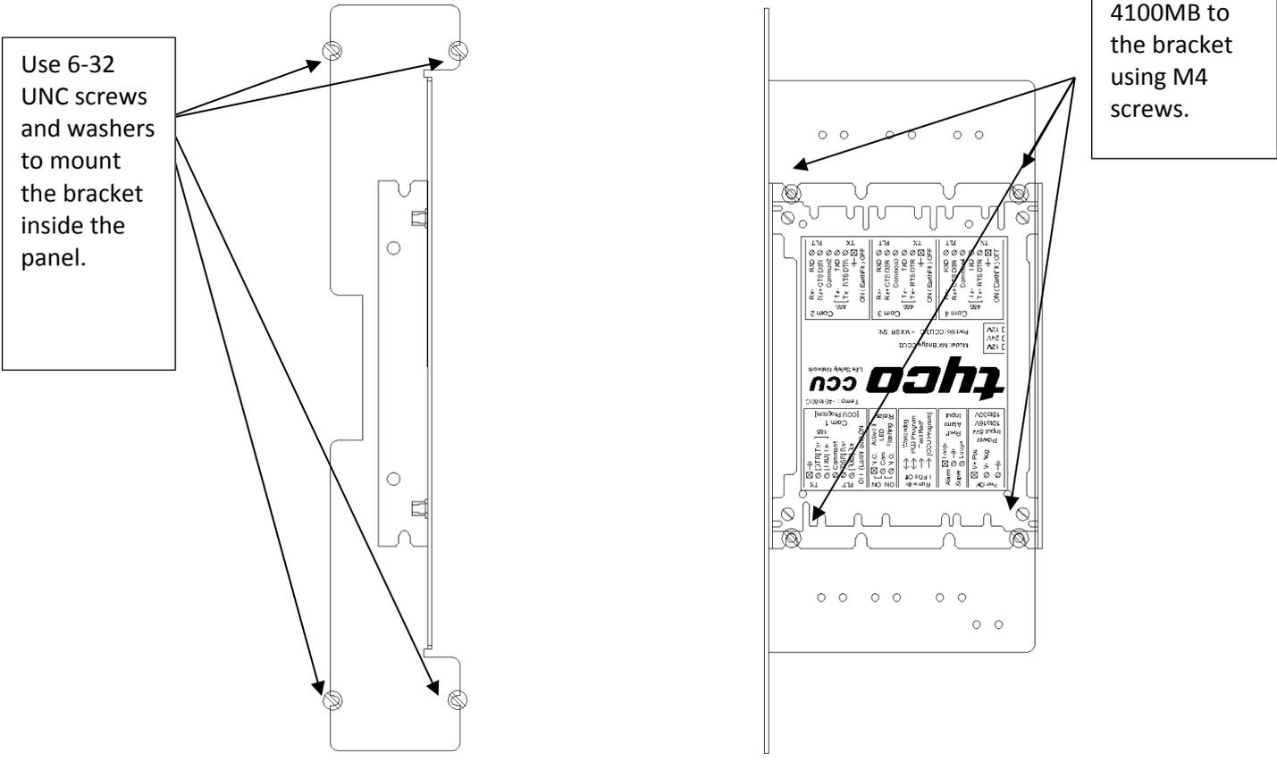
Figure 4: Mounting the 4100MB inside the Panel Enclosure
