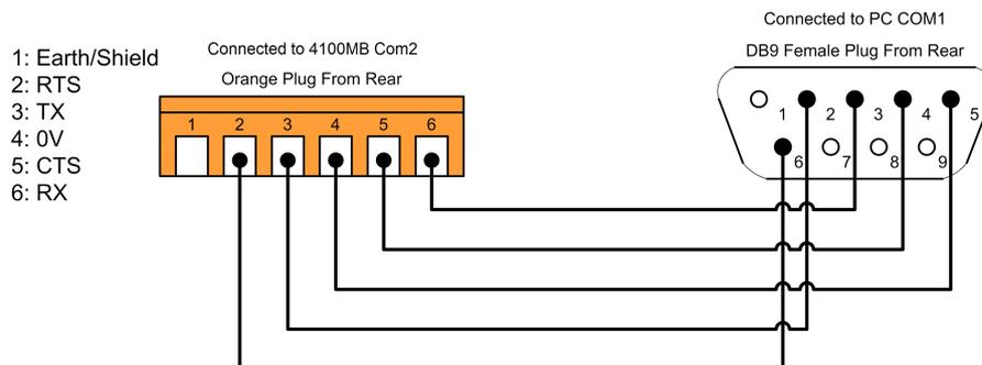
Figure 6: Connection between 4100MB and PC COM Port
