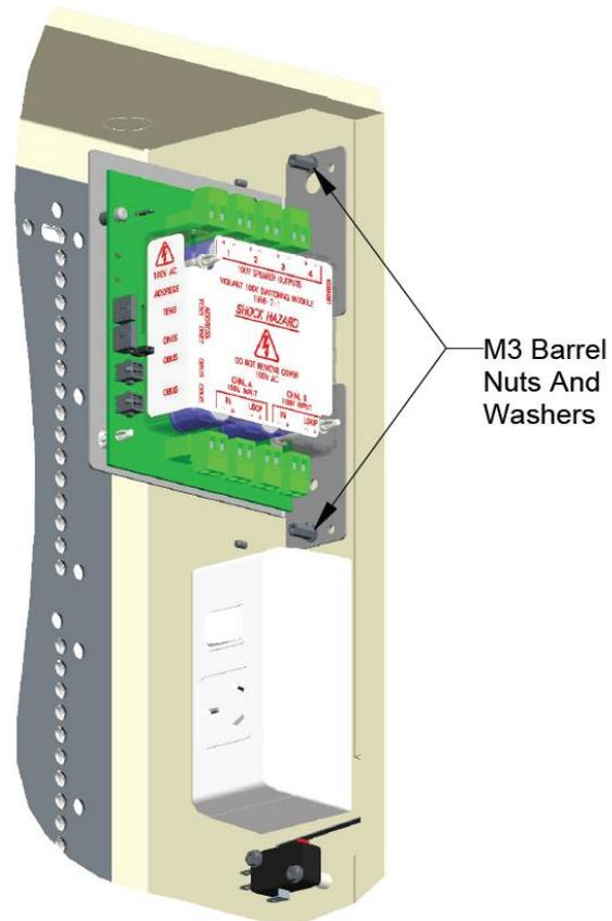
Figure 4 – 100V Switching Module in Slimline MX1 Cabinet
