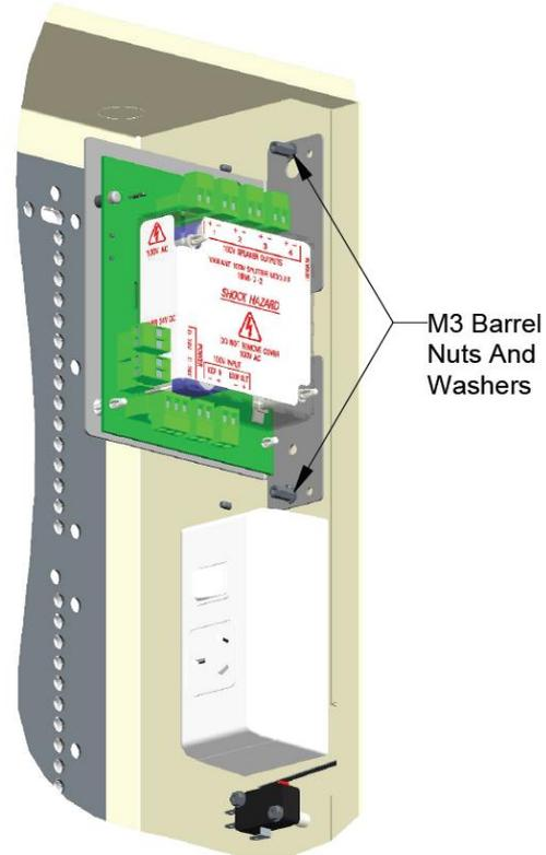
Figure 2 – 100V Splitter Module in Slimline *MX1* Cabinet
