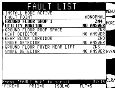
Figure 8-4. Fault List with Additional Missing Devices
