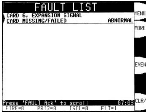
Figure 8-1. Sample Fault List Display Showing a Missing Card
