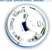
The 601SB Sounder Base provides a sounder function on conventional fire detection circuits. It operates independently of the detector circuit and may be used without an associated detector. When used without a detector, a sounder base cap should be fitted to cover the exposed terminals. The 601SB requires an external 24V dc supply and provides eight tones including the ISO8201T3 evacuation signal. It is identified by a green temporary park plunger.
