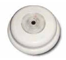
The Tyco 801F Flame detector is a digital addressable low cost infrared flame detector with some high-end features such as 'Solar Blind' operation for nuisance alarm-free reliability and an automatic detector health check feature. It will detect a 0.1m² flaming fire at a range of 20m. The 801F uses the standard range of *MX* detector bases and *MX* base accessories. An intrinsicaly safe version is available.
