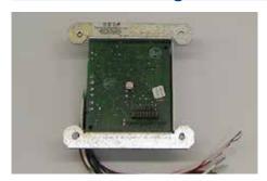
SIMPLEX AMZs provide an accurate, multi-featured 4-20mA interface for connecting analog sensors to Simplex addressable fire detection panels. The panel monitors the sensor and annunciates whenever a selected threshold level or fault condition is observed. Typical applications include: gas, air, liquid temperature, humidity, and air velocity sensing. The maximum distance from AMZ to a sensor is 1km. Each AMZ requires an address and up to 100 AMZs can be connected per panel.
