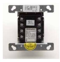
The 4090-9101 Zone Adaptor Module Monitor ZAM allows a 2-wire circuit of collective smoke or heat detectors to be interfaced on to the IDNet loop.
