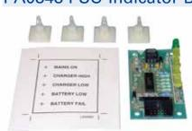
This PCB Assembly connects via a flat ribbon cable to the PSU24XX range of power supplies. The PCB provides optional Mains On, Charger Low, Charger High, Battery Fail and Battery Low LED indicators which may be mounted on the front facia of equipment. PCB Dimensions (mm): 75H x 40W x 30D. Supplied complete with self-adhesive PCB stand-offs and LED label. It mounts on 4 adhesivebased stand-offs, included with the PCB. Five Ø5.5-6mm holes need to be drilled at 10mm vertical spacing for the LEDs.
