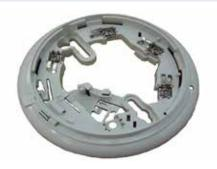
The 5B Universal Base contains no electronics and is suitable for indoor applications of both the 614 series collective (non-addressable) and 814 series analogue addressable detectors. It provides excellent space for cable access and terminations. Its larger skirt makes it suitable as a replacement for the earlier M614 base to cover any paint rims or for covering a larger hole in the ceiling. It features remote LED connections and an anti-tamper facility.
