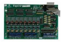
**FP0553**, F3200 8 Zone Input Expansion Kit Includes: PA0492, 8 Zone Module, LM0053 FRC, 8 x EOLR (std). (EOL = 2k7 5% 0.4W).
