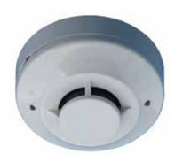
The P131A-Mk2 photoelectric smoke detector contains a state-of-the-art sensing chamber and analogue communication electronics. Used in conjunction with the VIGILANT MX4428 panel, the P131A-Mk2 has a high degree of false alarm immunity thanks to the advanced SmartSense algorithms.
