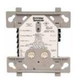
The ADCS130-Mk2 Supervised Relay Control Module provides a single switched supervised output on the MPR addressable loop. It supervises the output wiring for open or short circuit faults when the output is de-energised. The ADCS130-Mk2 can directly replace an ADC130 configured for supervised output operation (tabs in place).
