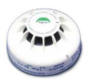
The MR601TEX has been developed to overcome the slower response of the optical detectors to hot burning fires, by increasing the sensitivity of the optical detector when it is associated with a rapid change in temperature. In this way it is intended to become a detector which can cover some of the risks currently covered by ion chamber detectors. Smoke detectors will not detect burning alcohol or other clean-burning liquids which do not generate smoke particles.
