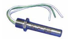
Constructed from stainless steel, the T54B is an extremely rugged heat detector that can be used to detect fires in the harshest of environments. The T54B can be used in environments with ambient temperatures up to 280°C and, being hermetically sealed, is impervious to most contaminants. The
