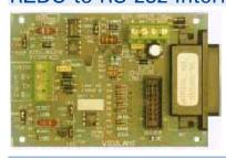
The RZDU to RS232 Interface is a small printed circuit board that converts Remote Zone Display Unit serial communications from a fire indicator panel into RS232 compatible signals. This module is required for an IO-NET Controller to receive information from an F3200/MX4428/F4000/ MX1 fire alarm panel.
