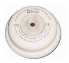
The 801FEx Intrinsically Safe Flame Detector forms part of the 800Ex Intrinsically Safe Series of MX Addressable Fire Detectors. The detector plugs into a 5BEx base. The detector is designed to transmit to a remote MX fire controller, digital signals which represent the infrared radiation produced by flaming fires involving carbonaceous materials. The 801FEx is a full featured flame detector for indoor applications. It must be connected via an EXI800 interface and galvanic barrier.
