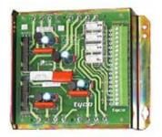
PA0792 TRAN9705-2 4x25W Transformer Module c/w Relays
