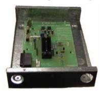
The IO-NET Programming Unit transfers the program to the IO-NET Controller PROMs. The Programming Unit is supplied complete with a cable to connect to a PC, the compiler programming software and the user manual.
