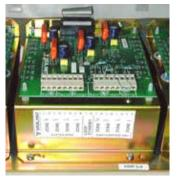
**PA0795** TRAN9706-1 4x10W Transformer Module without Relays
