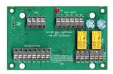
The MIO800 Multi-Input Output Module allows multiple input and output connections to be made between external equipment and the MX DIGITAL loop. Three inputs and two outputs are provided. Each input and output can be programmed independently to provide customised functionality.
