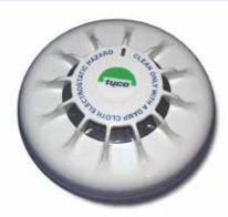
The 801PHEx Intrinsically Safe Optical Smoke & Heat Detector plugs into a 5BEx base. The detector is designed to transmit to a remote MX fire controller, digital signals which represent the status of the optical smoke and heat elements of the detector. Software within the controller interprets the returned optical and heat values to raise an alarm or other appropriate response according to the type of programmed configuration. The mode of detector may be:
