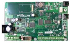
Configuration and diagnostics are performed from a standard PC web browser anywhere on the network. The PIB also provides remote across-network access to the diagnostic port of any panel directly connected to a PIB. It is supplied complete with Ethernet, MX4428 serial port, and I-HUB/panel FRC network port looms.
