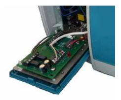
The VIO800 is an arrangement of the MIO800 Addressable Multi-I/O Module supplied ready to be fitted on to a VESDA LaserPLUS  $^{\text{TM}}$  or Laser SCANNER The MIO800's inputs and outputs are wired to the relay outputs and control inputs of the LaserPLUS or Laser SCANNER to allow compatible MX c.i.e. to monitor and control the VESDA units.
