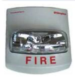
The 4906-910x Multi-Candela strobe is a high output xenon strobe capable of signalling evacuation using the ISO 8201 "T3" temporal pattern, as required by AS1670.4-2004 and AS 1670.1-2004. It produces white light with a link-selectable intensity of 15cd, 30cd, 75cd or 110cd. It is controlled by either the ISO 8201 Strobe Driver Module (PA1043) or a QE90 STRM Strobe Relay Module (PA0697). Note: A 24V output cannot be used directly.
