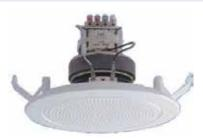
The 'One Shot' PA speaker and grille is designed to install easily into 10 to 13mm gyprock/plaster/ acoustic ceilings. Simply drill the required size hole, terminate the wiring and push the speaker into the ceiling until it snaps into place. They are designed to meet the requirements of AS2220.1, with a transformer cover (not shown in the image) and 22µF capacitor. The transformer has 5 power taps from 0.33 to 5W and a 4 way terminal block.
