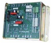
**PA0794** TRAN9705-4 2x25W Transformer Module c/w Relays
