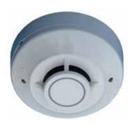
The T131A-Mk2 heat detector is a state-of-the-art dual thermistor heat detector with analogue communication electronics. Used in conjunction with the VIGILANT MX4428 panel, the T131A-Mk2 has a high degree of false alarm immunity thanks to the advanced SmartSense algorithms. It is panel programmable to either Type A (with Rate Of Rise) orType B (fixed temperature only) to maximise system design flexibility.
