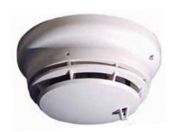
TrueAlarm multi-sensor 4098-9754EA combines the TrueAlarm photoelectric smoke sensor with a fast-acting and accurate TrueAlarm thermal sensor to provide both features in a single sensor/base assembly. Analog information from each sensor is digitally communicated to the control panel where it is analysed.
