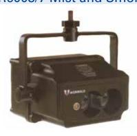
The IR6003 Beam detector is an intelligient device that has been designed to monitor a large area containing plant or equipment. The IR6003 can be supplied in different configurations to suit mist and smoke type hazards. The waterproof housing has an easy to fit bracket that allows simple installation and commissioning. The fascia of each unit has been equiped with an LED that flashes on fault condition and indicates steady on alarm.
