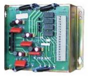
**PA0796** TRAN9706-2 4x10W Transformer Module c/w Relays
