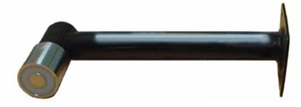
The EAO411 Electromagnetic Door Holder is designed to hold fire and smoke doors open under normal conditions, but automatically close under their own spring return mechanism when a fire or smoke alarm system is activated. The door is held open by the magnetic force between an
