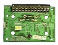
The DIM800 Detector Input Module interfaces two collective detector circuits onto the MX addressable loop.
