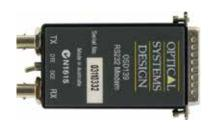
The OSD 139AF Asynchronous RS232 Transceivers can interconnect one RS232 data channel over 3km of multimode fibre (OSD139AF) or over 50km of singlemode fibre (OSD 139AFL). These can provide complete end-to-end isolation of a full duplex asynchronus data transmission at up to 60kbps.
