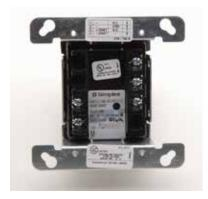
The 4090-9002 Relay IAM allows the CIE to control a remotely located Form "C" Relay contact using IDNet addressable communications for both data and module power. Typical applications are for switching local power for control functions such as magnetic door holders, or control of HVAC components, pressurisation fans, dampers, etc.. Relay contact status is also communicated to the CIF. The address is set by DIP switch under the resealable
