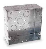
Boxes for mounting Zone Adaptor Modules (ZAMs) are available in 2 sizes. Both boxes are of welded steel construction, galvanised for corrosion protection. The ZAM boxes both feature round and eccentric knock-outs for cable entry on each surface
