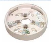
The **Z131A** Detector Base should be mounted on a flat surface with suitable fasteners. A tamper-resist feature is incorporated in the base which, when used, prevents removal of the detector without using a small screwdriver or similar tool.
