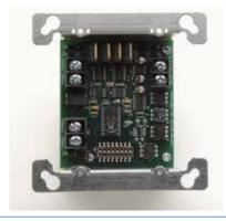
The 4090-9117 Power Isolator provides monitoring and short circuit protection for 24Vdc power wiring to IDNet addressable devices. In the event of a short circuit, it opens a two-pole electronic switch, isolating both power circuit conductors. This function can also be selected from the CIE. The isolator reports to the CIE. when it is in isolation mode. It also reports the extent of shorted wiring by identifying the addresses of non-communicating devices
