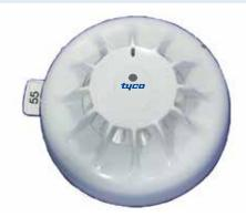
The 814H is a flexible cost-effective addressable heat detector with most of the features of MX VIRTUAL detectors. The 814H returns the temperature to the MX fire alarm panel which allows various detection modes, including all AS 1603.1 Types and many AS 7240.5 classes to be implemented. The 814H uses a high quality thermistor with very low thermal mass. This allows the detector to function as a heat detector as well as providing a fast and accurate temperature display.
