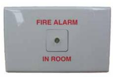
The E500 Mk2 range of latching remote indicators provide latching remote indication of an alarm condition on a fire detector. They are used typically where a T54B probe type fire detector is installed (which may be in an inaccessible location), and indication of alarm must be provided in an easily accessible area. For example, where the detectors are in roof spaces or cupboards, exhaust hoods etc and indication is required in the room or corridor.
