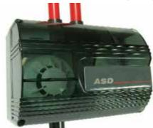
The ICAM IAS Air-Sampling Smoke Detection system provides a flexible detection solution to meet the needs of numerous applications. The IAS systems actively draws air from the protected area through sampling holes in a pipe network. Sampled air is filtered and then analysed by two *MX* detectors. The IAS system is available as a twin inlet pipe configuration (IAS-2), and can be fitted with two detectors per system. Flow failure is reported as a device fault via an *MX* MIM800 module.
