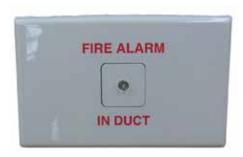
The E500 Mk2 range of remote indicators provide remote indication of an alarm condition on a fire detector. They are used where the fire detector is installed in an inaccessible location, and indication of alarm must be provided in an easily accessible area. For example, where the detectors are in roof spaces or cupboards, under the floor, or in hotel rooms, and indication is required in the room or corridor
