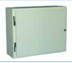
FP0804 comprises a power supply for MX4428 mounted within the FP0576 8U battery box which has a similar finish to the range of standard VIGILANT 19" rack cabinets. The cabinet provides IP51 protection and the door is secured with a 003 lock. Use with indicator PCB, PA0848 for LED indication on the cabinet door of Mains On, Charger Low, Charger High, Battery Fail and Battery Low.
