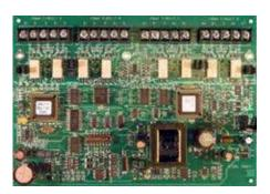
The IDNet+ is an enhanced IDNet loop card suitable for use in SIMPLEX 4100ES and 4100U systems. It has inbuilt addressable short circuit isolators which can be configured to provide up to four isolated loops or 8 spur circuits.
