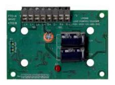
The LPS800 Loop Powered Sounder Module switches up to 75mA @24V dc to activate external notification devices. The module is capable of monitoring and signalling Normal & Short or Open circuit condition on the sounder circuit. The LPS800 short-circuit protection prevents a single short circuit condition from disabling more than the output containing the short-circuit. The LPS800 LED reports status to the user.
