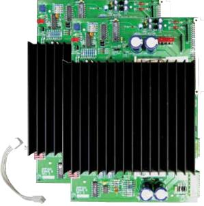
**KT0519** 200W Amplifier Module Kit The 200W amplifier comprises two PA0647 AMP200 PCB modules and one LM0141 FRC
