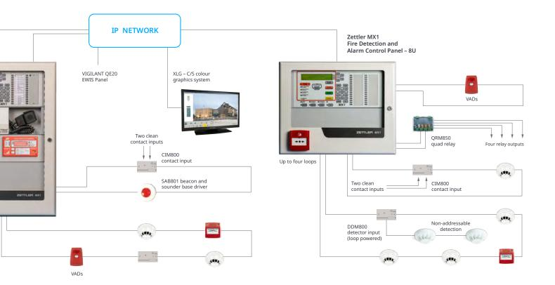
functions and timers, programmable outputs for warning devices and ancillary controls makes the MX1 configurable to almost any fire detection requirement. The panel's site-specific database is duplicated, reducing downtime and increasing reliability.
