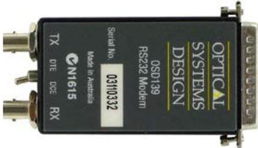
The OSD139HS Asynchronous RS232 Transceivers can interconnect one RS232 data channel over 3km of multimode fibre (OSD139HS) or over 40km of single mode fibre (OSD139HSL). These can provide complete end-to-end isolation of a full duplex asynchronous data transmission at up to 120kbps. The OSD139HS are high performance fibre optic modems capable of linking asynchronous RS232 data over several kilometres at speeds ranging from DC to 120kbps. Recommended for I-HUB Ring network applications.
