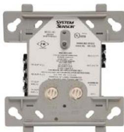
The ADM130-Mk2 is an addressable input module that allows the connection of hard contact detection devices. The module's two wire input is supervised for faults. An LED indicator allows visual monitoring of the module's status. An output is provided for connection to a remote LED indicator. Suitable remote indicators allow visual indication of the module's alarm status
