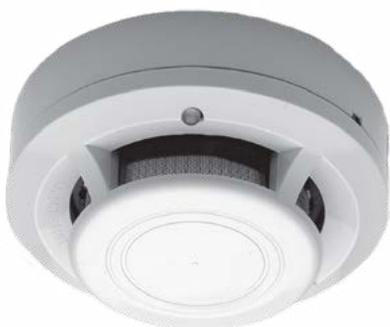
The P132A Addressable Laser Smoke Detector is a very high sensitivity smoke detector that utilises a laser photoelectric sensing chamber, providing significant improvements in signal-to-noise ratio compared with an LED light source. The detector is designed to provide open area detection for clean environments, or cubicle detection for high value equipment. The P132A Laser mounts to the B501AUS base or B200SR Sounder Base.
