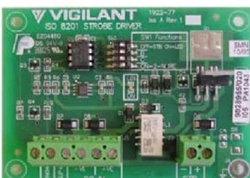
The ISO 8201 Strobe Driver generates an ISO 8201 compliant "T3" pattern for the Multi-Candela strobe 4906-9104. It connects directly to a supervised relay output of a fire alarm panel and drives one or more lines of strobes with a synchronised T3 pattern. The fire alarm panel's output supervision supervises the wiring from the panel to the strobes. The output signals of up to 5 modules can be synchronised. Four standoffs are supplied for mounting.
