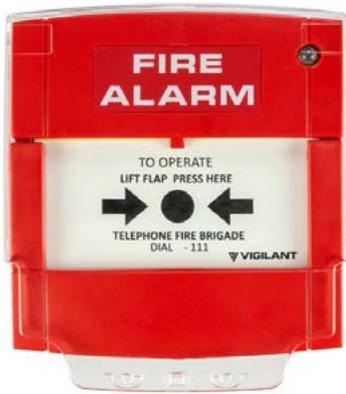
The VNCPI is a conventional indicating manual callpoint (MCP) that is suitable for indoor applications. It is supplied with a plastic element, which deforms when pressed in to release a microswitch.
