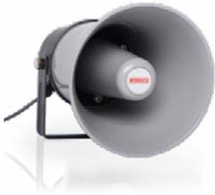
The EA0020 is a high performance 8 ohm horn speaker for use in smaller PA applications requiring a low impedance audio solution. It is ideal for use as an external sounder for the VIGILANT IP65 AVI Mk2 where increased warning tone volume is required. The EA0020 should be mounted adjacent to the IP65 AVI Mk2. The cable supplied with the speaker should enter the AVI using the supplied 16mm cable glands and be terminated at the AVI Controller board.
