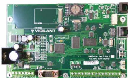
Configuration and diagnostics are performed from a standard PC web browser anywhere on the network. The PIB also provides remote cross-network access to the diagnostic port of any panel directly connected to a PIB. It is supplied complete with Ethernet, MX4428 serial port, and I-HUB/panel FRC network port looms.
