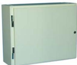
This battery box provides 8U of 19" rack capacity and has a similar finish to the range of standard Vigilant 19" Rack Cabinets - 1.6mm mild steel construction, with powder coated, cream wrinkle finish. The cabinet provides IP51 protection and door is secured with 003 lock. 24 volt battery capacity is 80Ah using 2 x PS-12800 batteries (not stocked) or up to 120Ah using 6x 40Ah batteries (BA12400).
