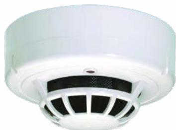
The 4351E thermal detector incorporates an Application Specific Integrated Circuit (ASIC). Combined with the latest in thermal element technology the detector provides efficient and accurate detection of fires, especially in environments such as boiler houses or kitchens where smoke detectors are inappropriate due to the high level of airborne contamination. The 4351E operates when the detected temperature exceeds 78°C.
