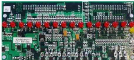
The VIGILANT LED-RZDU (PA1048) is a Remote Zone Display Unit (RZDU) that provides a flexible and cost-effective “building block” for the construction of remote LED/mimic displays for VIGILANT fire alarm panels equipped with an RZDU port. It is highly configurable, with a range of mounting options for front or rear service, and is compatible with a variety of LED display and mimic termination boards.
