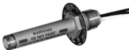
DETECT-A-FIRE thermal detectors are UL Listed, and FM Approved detection and release devices used with fire detection systems to activate alarms and actuate extinguishing systems. This Rate Compensated device combines the best features of both fixed temperature and rate-of-rise detectors. Contacts open on alarm.
