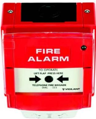
It is supplied with a plastic resettable element, which deforms when pressed in to release a microswitch. The element is not destroyed and can be reused many times by resetting the MCP using the test/reset key provided. A clear plastic cover, which must be lifted to gain access to the element, provides protection against accidental activation. The MCP is easily tested using the test/reset key.
