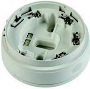
The 80DSB is an indoor detector base specifically for use with the MX addressable detectors. The base incorporates a sounder that is activated directly by the detector plugged into the base.
