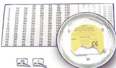
The 800 Series detectors incorporate a feature which automatically transfers the address flag to the detector base when the detector is plugged into the base. On removal of the detector the address flag is retained in the base, thus helping to ensure that detectors are not accidentally returned to the wrong detector base following service routines. Address flags are supplied in packs of 100.
