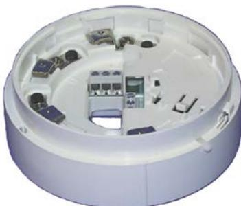
The 814RB Addressable Relay Base provides two sets of changeover volt-free relay contacts capable of switching 1A (resistive) @30Vdc. The relay function is controlled by the MX fire alarm panel via the detector fitted to the 814RB. The 814RB may be mounted directly to the ceiling or plugged into a 4B/5B, Universal or 4B-I/5B-I Isolator Base.
