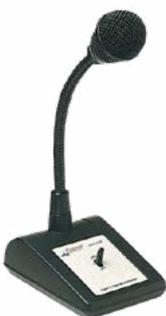
The SU0169 Desktop Paging microphone is a dynamic microphone with a cardioid polar pattern. It features a short-off press-to-talk (PTT) switch with an open-off type extra switch. It has low handling noise and a 600 ohm balanced output impedance. Compatible with the FP0539 Paging Console.
