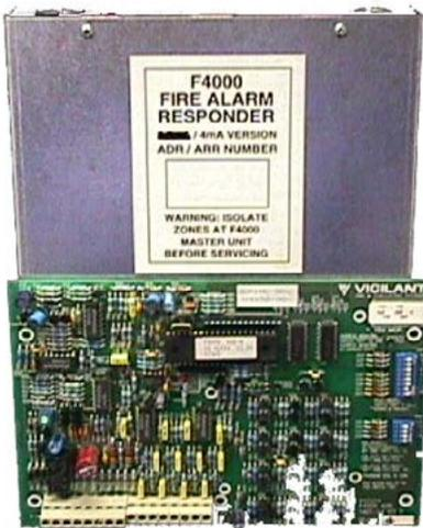
The PA0497 version of ADR is the only version suitable for general use in New Zealand. It supports four "smoke" circuits with short circuit defect. Indicating heat detectors are compatible with modification - refer to LT0126.
