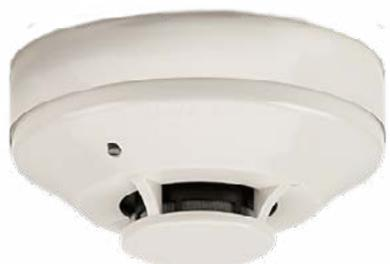
The P135A/2251TMB is a photoelectric smoke detector with supplementary 57°C thermal. The ACCLIMATE uses advanced on-board software to combine the signals from the photo and thermal elements. This software creates a true multicriteria detector capable of rejecting nuisance sources, but still responding quickly to real fires. It has the capability of adjusting its sensitivity according to the type of environment that it is installed in.
