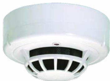
The 2351TEM photoelectric smoke/thermal detector incorporates an optical chamber and a thermal element, which in turn are continually monitored by an on board processor using algorithms developed specifically for the unit. An alarm signal is only enabled in the detector once the processor is satisfied that an incipient fire has been detected. By using a combination of inputs, the incidence of nuisance alarms is reduced while at the same time, the response time to an actual fire is also improved.
