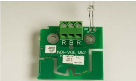
The Indi-VIGIL Indicating Module, when installed in a manual call point or wired to a clean-contact detector, is compatible with VIGILANT fire alarm systems in the same quantities as the indicating manual call point and Indi-VIGIL heat detector.
