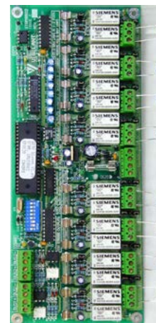
FP1070 STRM9502 (PA0697) Strobe/Relay Module (WEB) with AS 2220/ISO 8201 Selection
