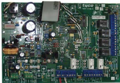
PA0873 , F3200 AS4428 MAF/PSU 3A 1931-3-3 Size: 160 x 250 x 45 mm, 400g
