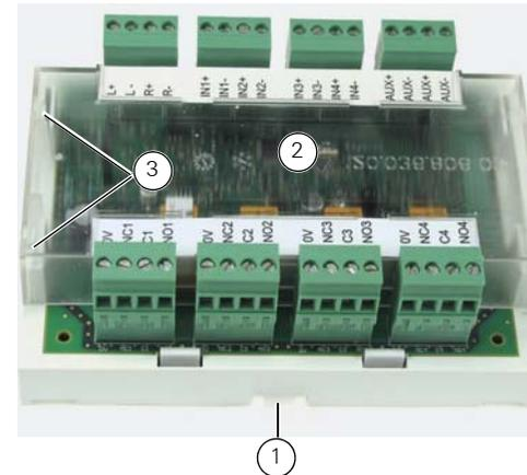
Fig. 1: QIO850 Quad Input/ Output Module
