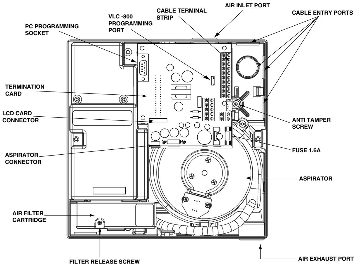
**Fig. 3 VLC-800MX Component Location**
