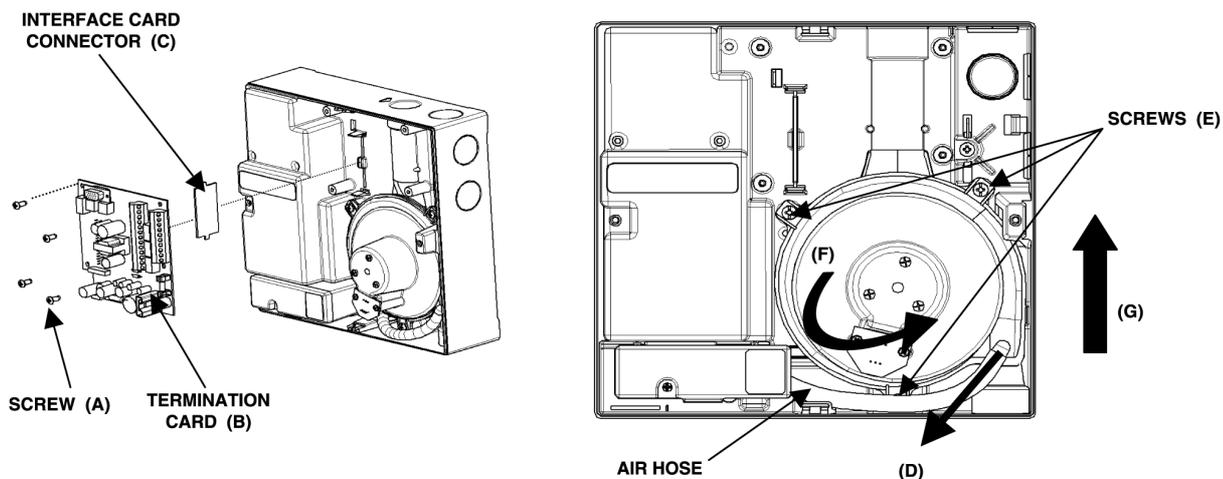
Fig. 16 Removal/Replacement of Aspirator Assembly
