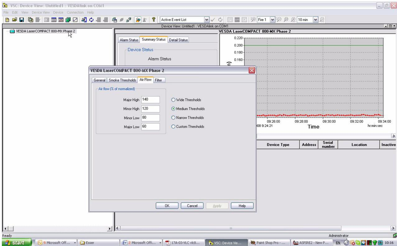
**Fig. 13 Flow Threshold Setting**
