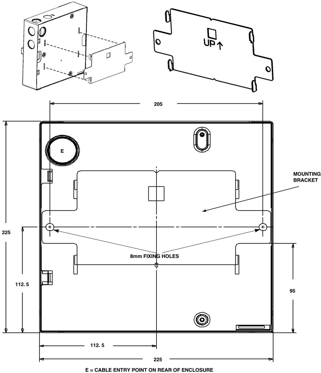
Fig. 8 VLC-800 Mounting Bracket
