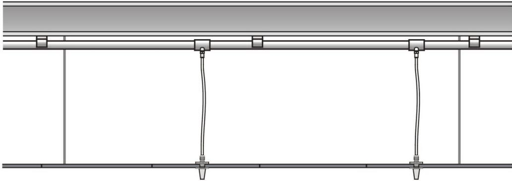
**Fig. 7 Capillary Sampling**
