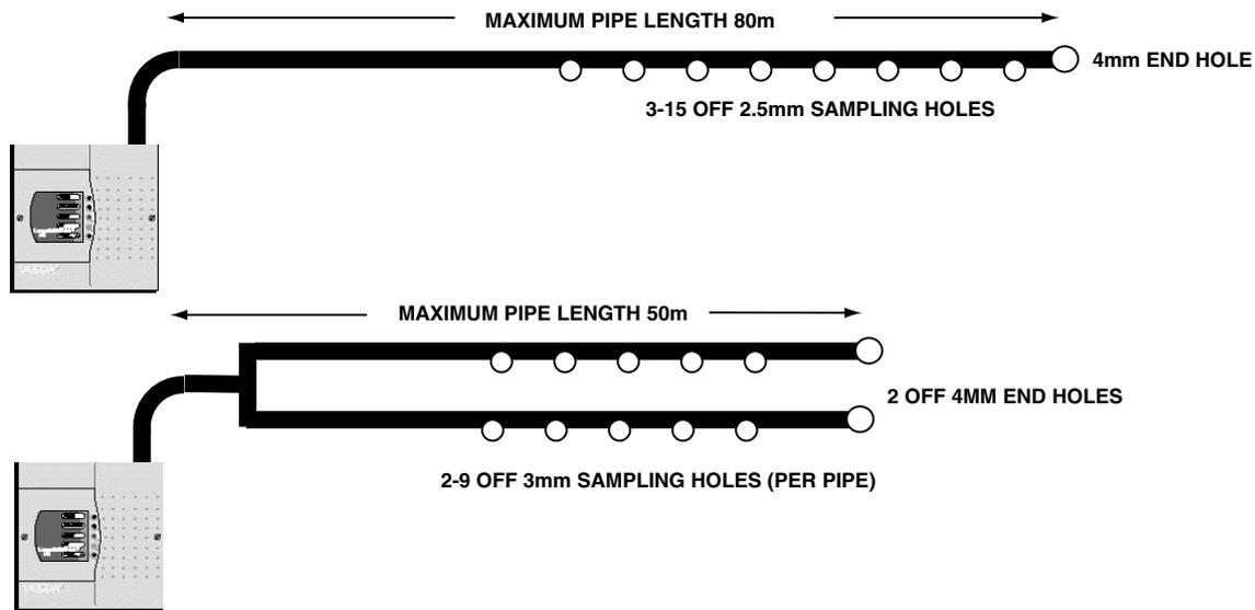
Fig. 6 Pre-engineered Pipework Configurations
