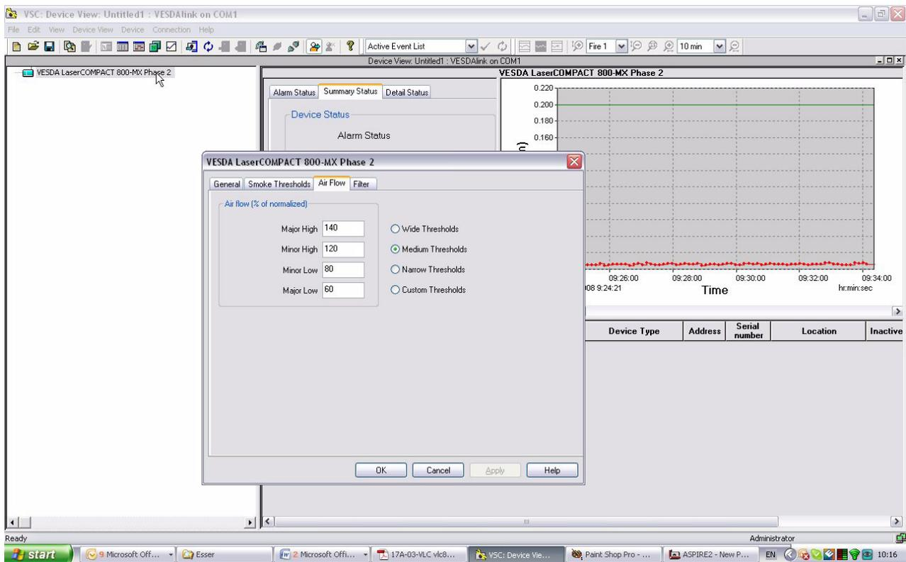
**Fig. 13 Flow Threshold Setting**
