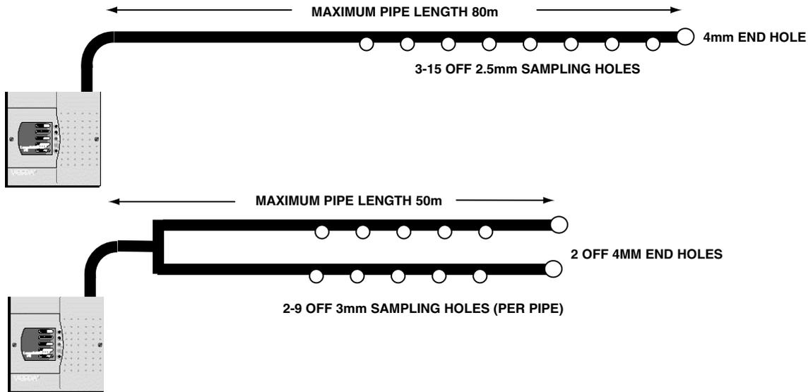
**Fig. 6 Pre-engineered Pipework Configurations**
