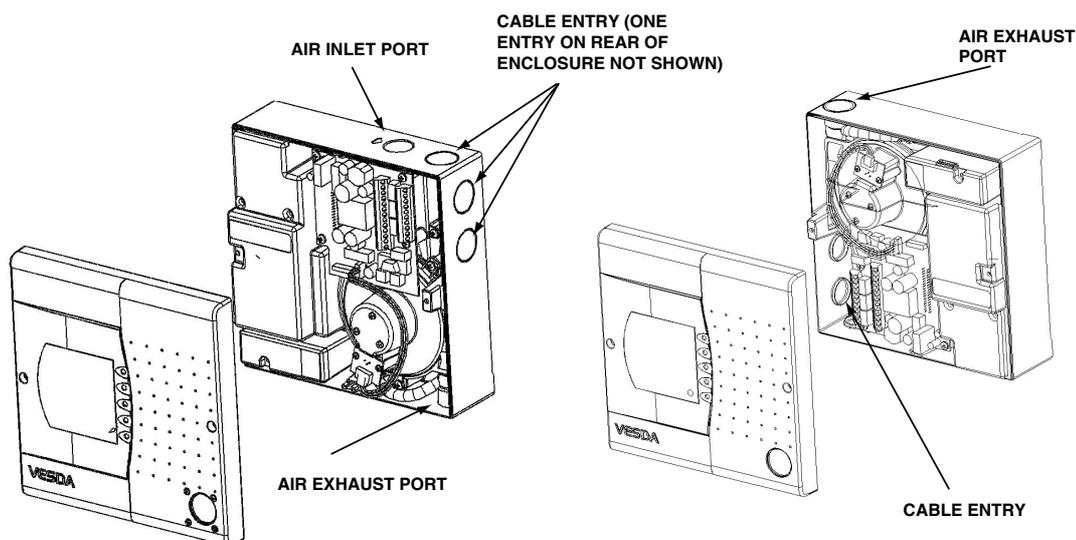
**Fig. 9 Detector Orientation (the backbox shows the generic termination card)**
