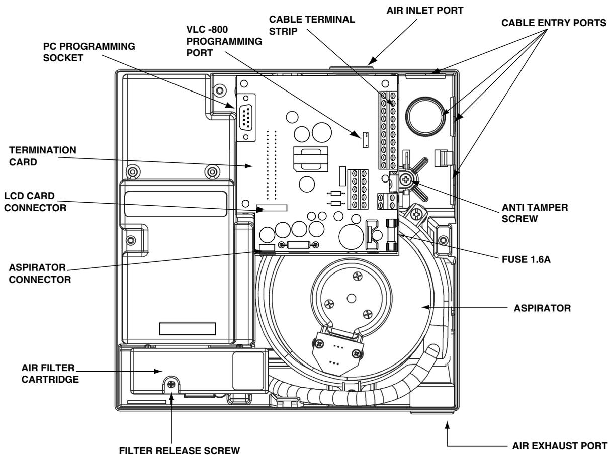
**Fig. 3 VLC-800MX Component Location**
