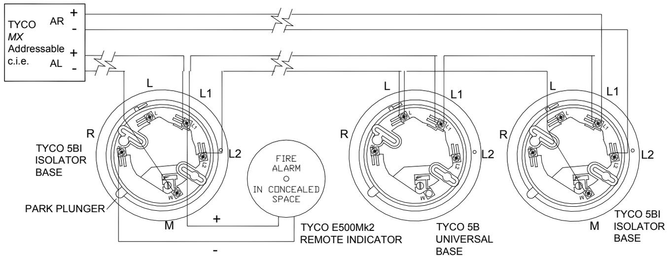
The MX c.i.e. can be programmed to illuminate a Remote Indicator for detectors in alarm other than the detector base to which the Indicator is connected.
