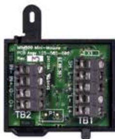
The MIM800 Mini Input Module monitors a voltage-free contact and transmits its state to the CIE. It can be programmed to monitor either Normally Open (default) or Normally Closed contacts. The MIM800 can be programmed to monitor:
