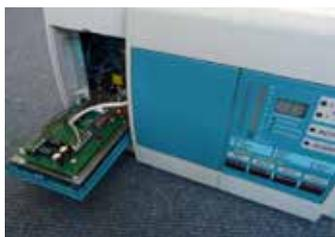
The VIO800 VESDA Interface Module is an arrangement of the MIO800 Addressable Multi-I/O Module. The MIO800 is supplied fitted on to a mounting bracket suitable for installation within all models of VESDA LaserPLUS or a LaserSCANNER which have relays fitted. The MIO800's inputs and outputs are wired to the relay outputs and control inputs of the LaserPLUS or LaserSCANNER to allow the compatible MX CIE to monitor and control the VESDA unit (VESDA not included). Wiring is not included.
