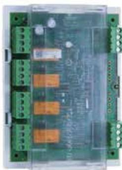
The Quad Relay Output module provides four voltage-free change-over relay outputs or switched auxiliary supply (24V/48V selectable) outputs. Supervision of the auxiliary supply can be enabled to detect disconnection or failure. The QRM850 includes an MX loop short-circuit isolator and can be programmed using the IR link from the 850EMT.
