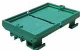
The DIN Rail Mounting Kit provides a convenient way to fix the large format modules (72 x 110mm) onto a standard DIN rail for in-cabinet installations. The MIO800 Module is fitted to the Mounting Kit by sliding the two Base elements onto the MIO800 PCB. Two foot elements are then attached into slots on the bottom side of the Base elements. Finally slide two Side elements onto the ends of the Base elements.
