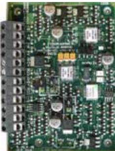
The DDM800 Universal Fire & Gas Detector Module is designed to monitor and signal two conventional 2-wire 20V fire detector circuits (or two 4-20mA current loop sensors on MX4428). It can be loop powered for certain applications - especially the low-voltage (LV) mode using the VIGILANT 614 smoke and heat detectors, or powered from an external 24V supply to provide a wide range of detector compatibility including intrinsically safe (IS) detectors and reduced *MX* loop loading.
