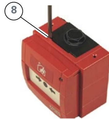
Remove the four fixing screws used to lock the call point to the back box.
