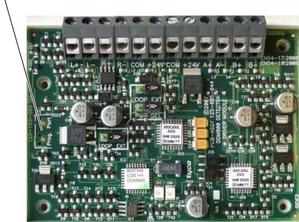
Fig. 1: DDM800 – Universal fire and gas detector module
