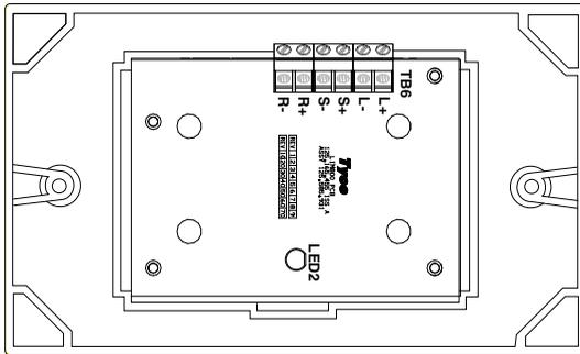
Fig. 4: LIM800 Fitted to Cover
