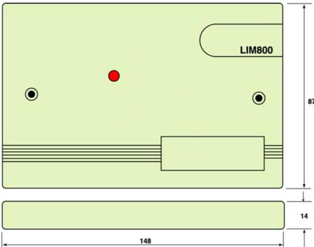
Fig. 7: LIM800 Line Isolator Module Facia Plate
