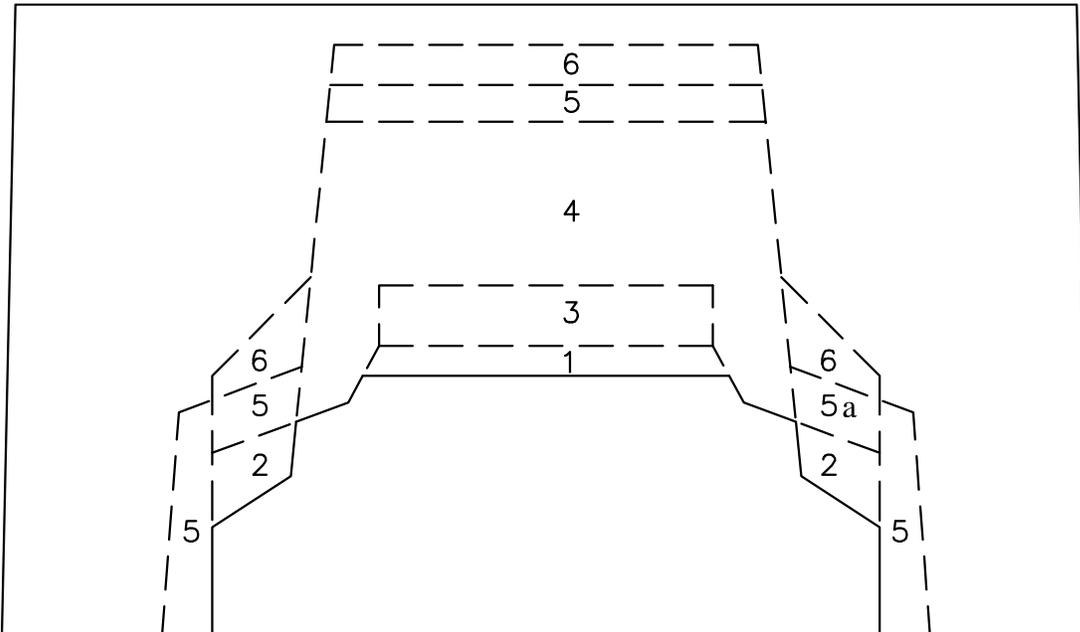
The following sections must be removed from the Universal Baffle to fit the profile of the respective detectors. Sections are removed by cutting or tearing along the perforations.
