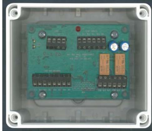
Fig. 3: MIO800 Mounted in D800 Housing
