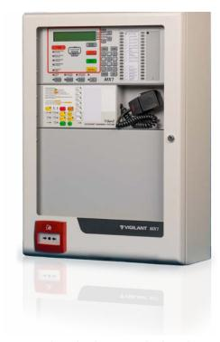
For non-emergency paging, the front panel microphone can be combined with the 4 area PA/Paging push-buttons and one or more FP1117 100V Switching modules connected to the T-Gen2 100V output to enable voice announcements to be selectively made to different areas of the building.
