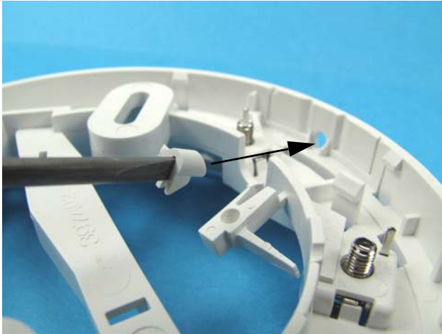
Fig. 4: Inserting the LED aperture plug
