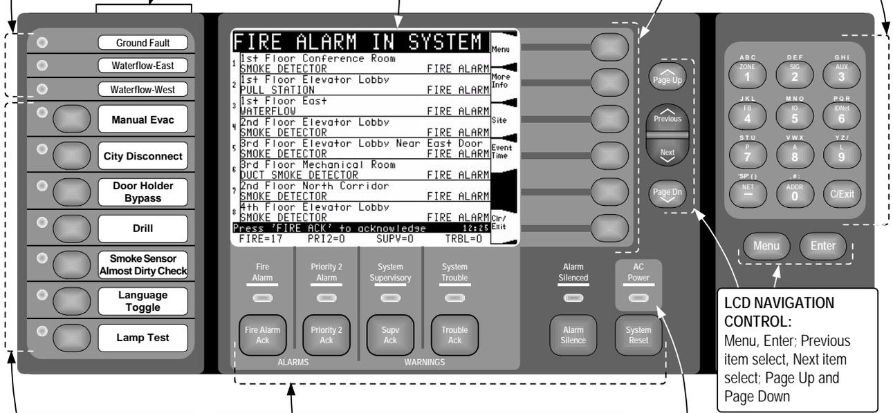
**SEVEN PROGRAMMABLE FUNCTION SWITCHES**, each equipped with dual color LED indicators; the top six LEDs are selectable as either red or yellow, the bottom LED is selectable as either red or green; **NOTE: Program the bottom switch as "Lamp Test" for UL listed systems**
