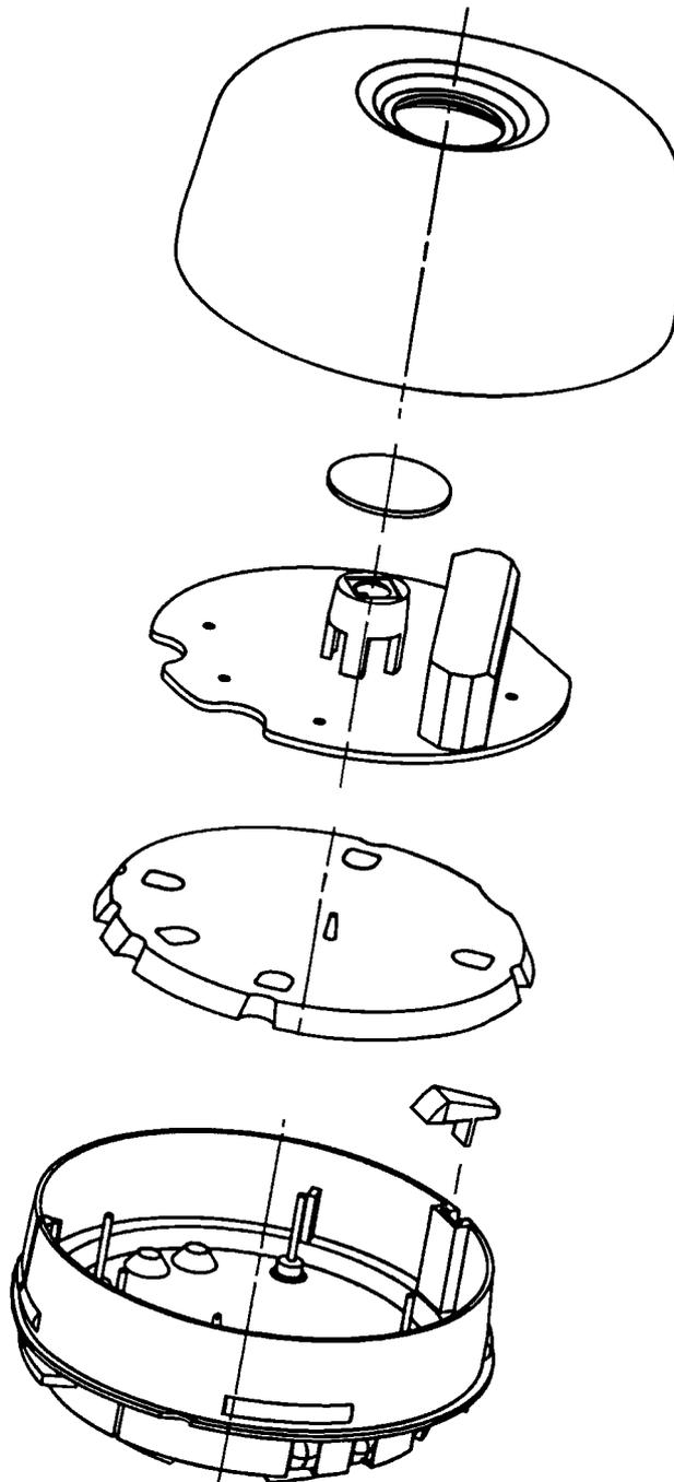
**Fig. 3 General Assembly, Type MS302Ex Flame Detector**
