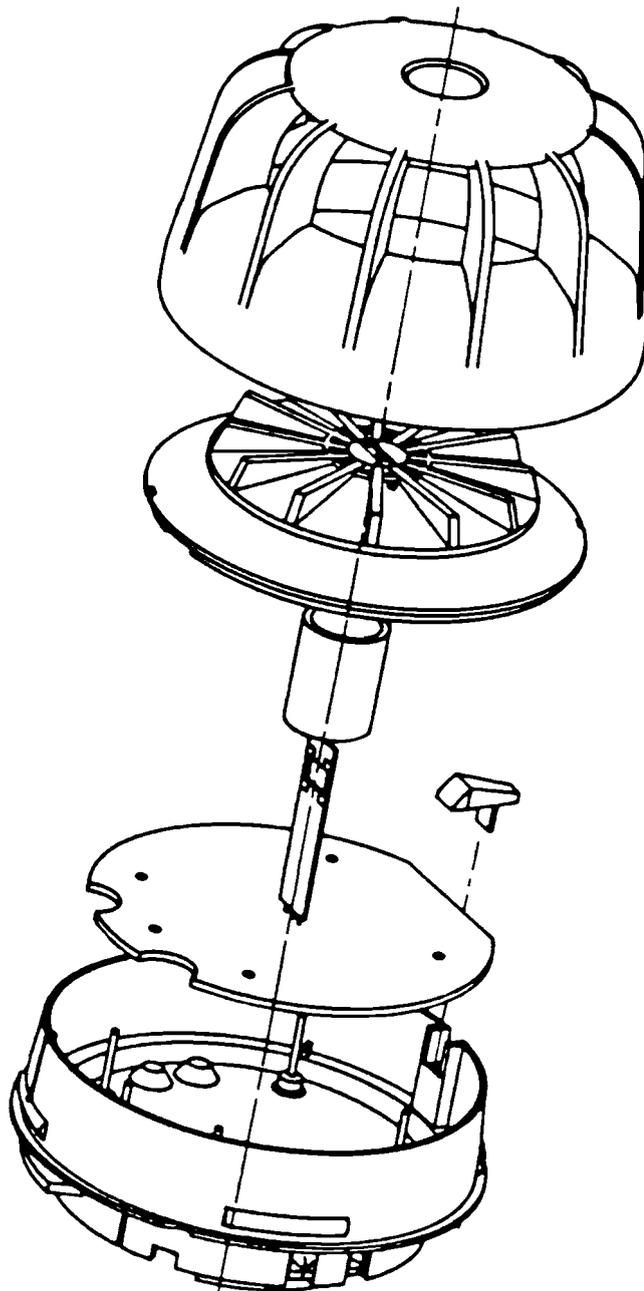
Fig. 2 General Assembly, MD300 Heat Detector
