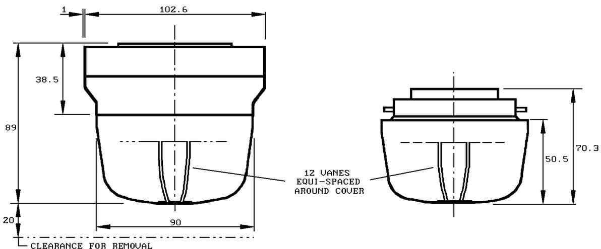
Fig. 3 Overall Dimensions MD300 Detector Range
