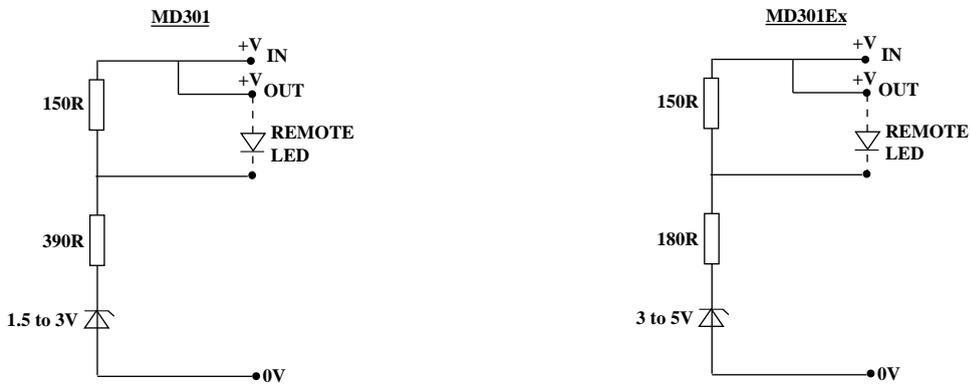
**Fig. 4 Alarm Load Presented to the Controller by the Detector**
