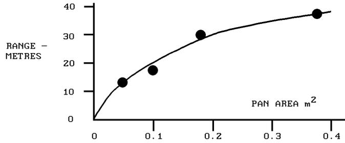
Fig. 4 Detector Range vs Pan Area - Petrol
