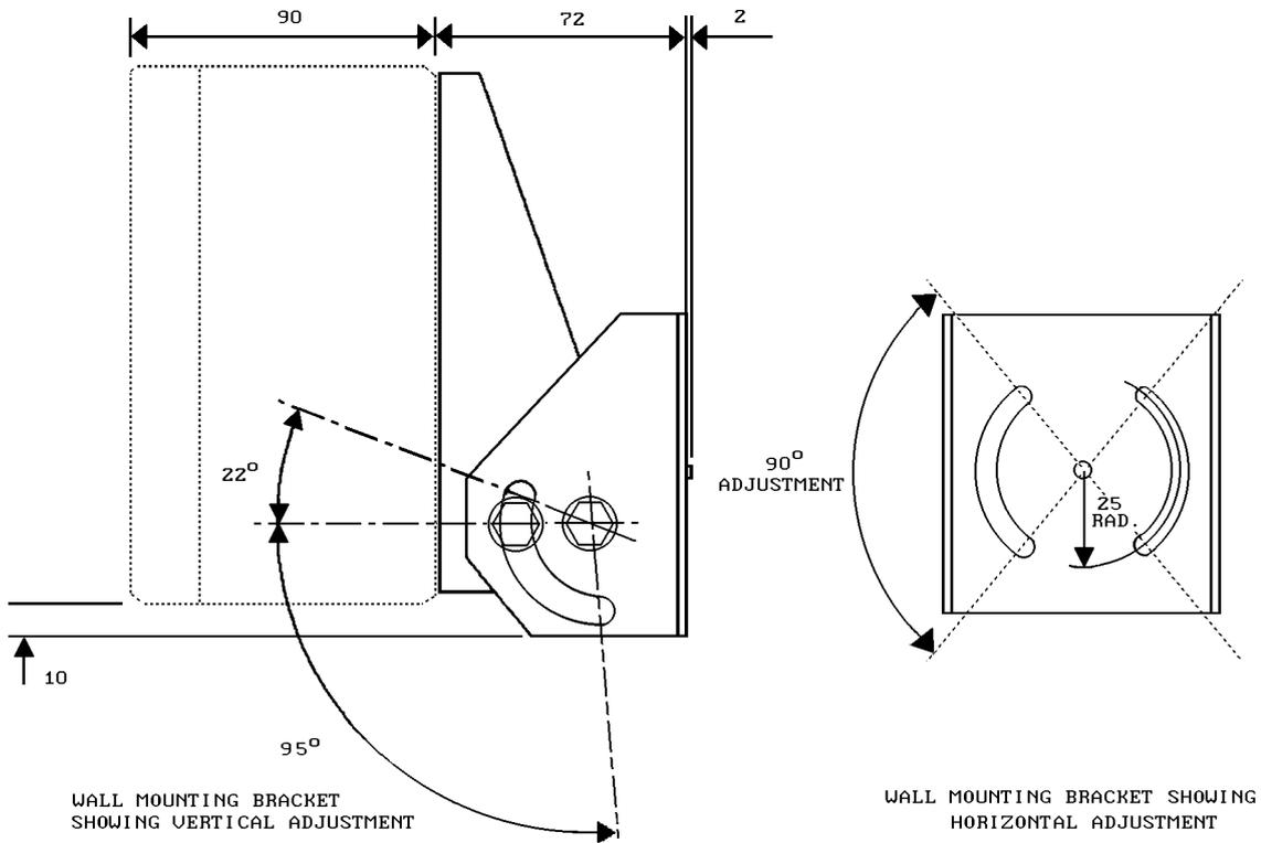
Fig. 6 Mounting Bracket [Type B Not Stockcoded]
