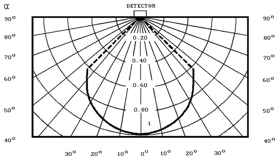
**Fig. 9 Relative Range vs Angle of Incidence**
