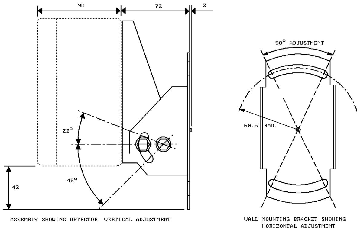
**Fig. 5 Mounting Bracket [Type A Stockcode 517-001-184]**
