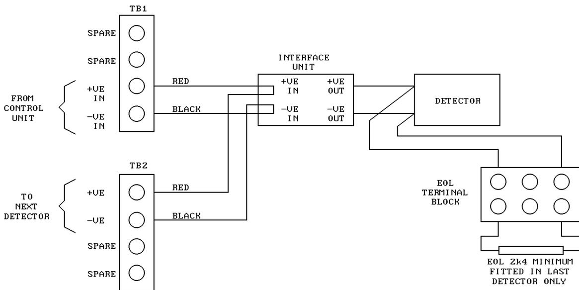
Fig. 4 S161 Connection and Internal Wiring Including EOL
