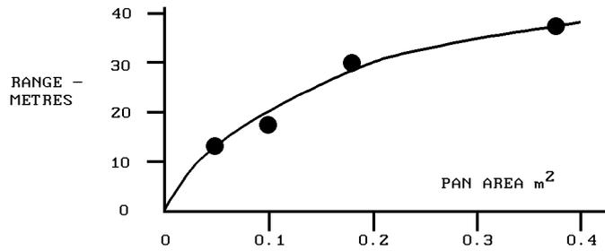
Fig. 8 Detection Range vs Pan Area - Petrol
