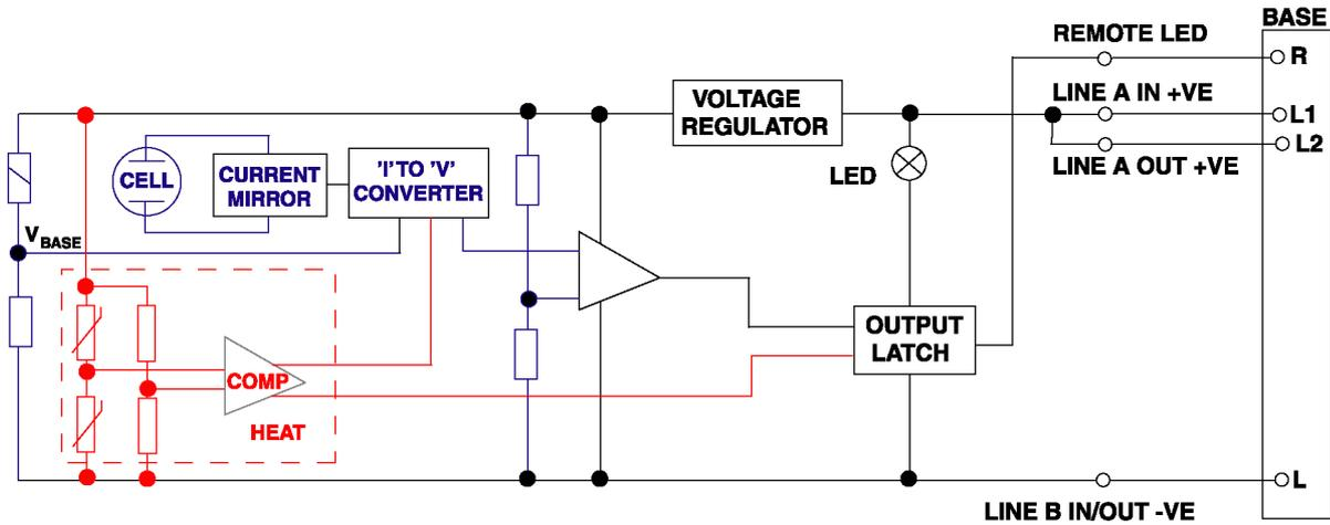
Fig. 2 Simplified Block Schematic Diagram of Detector
