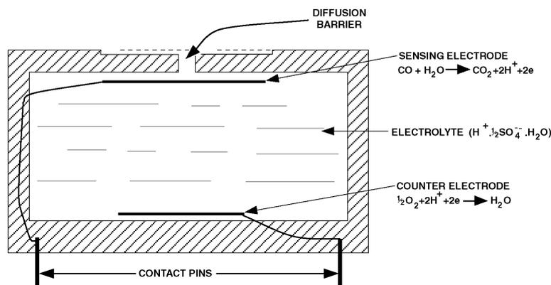
**Fig. 1 Representational Diagram of CO Sensing Cell**
