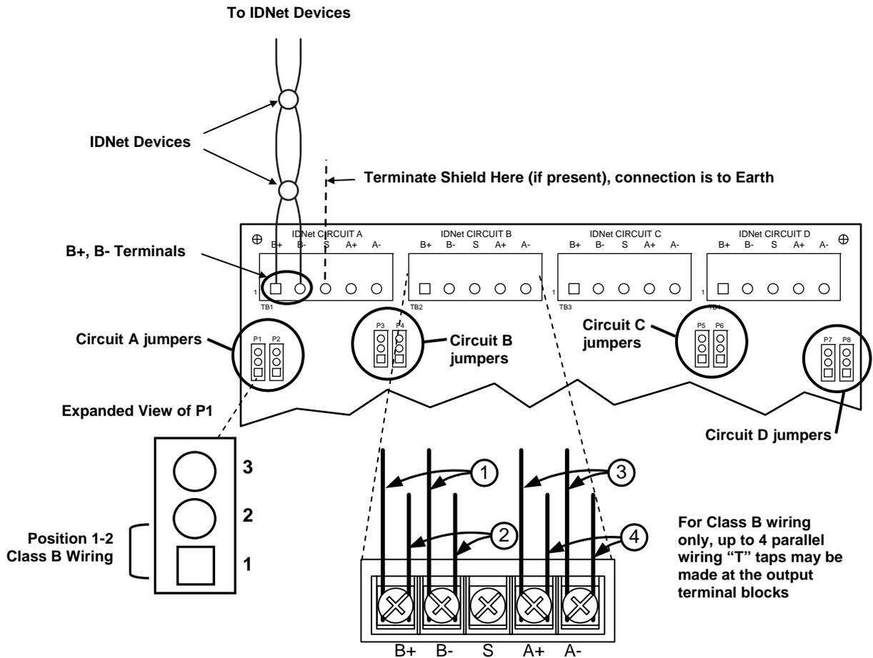
Figure 6. Class B Wiring
