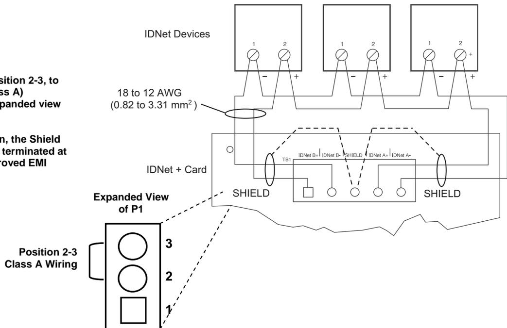
Figure 5. Class A Wiring (Shield Optional)
