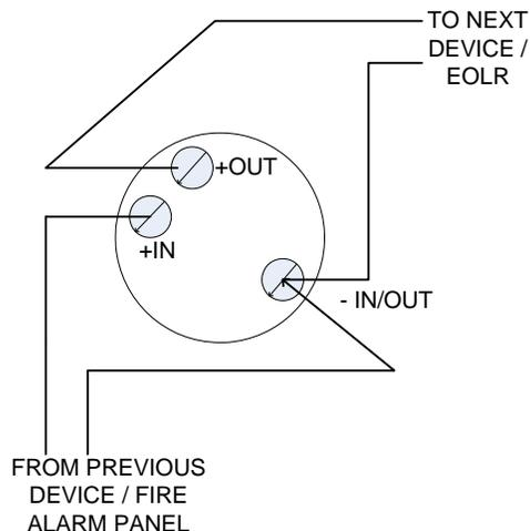
**Figure 7. Typical Detector Wiring**
