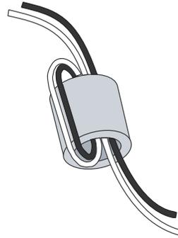
Figure 4. Ferrite Bead
