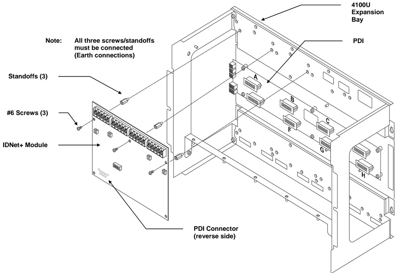
**Figure 2. Mounting onto the Power Distribution Interface (PDI) (4100U Shown)**
