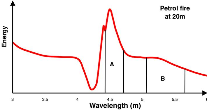
**Fig. 4 Measured Flame Spectral Characteristics**
