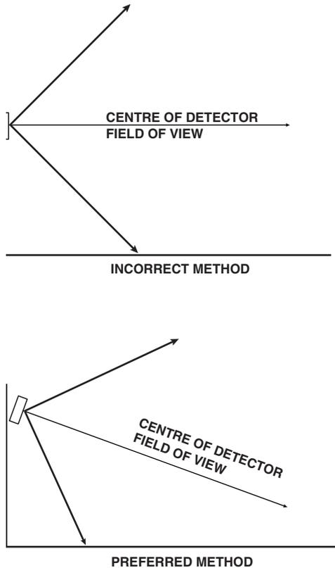
**Fig. 24 Detector Orientation Relative to Horizon**
