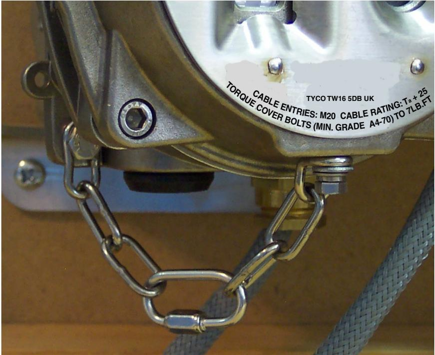
**Fig. 32 Safety Chain Connection**
