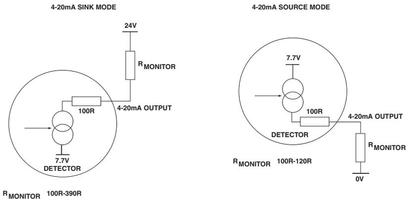
**Fig. 7 4-20mA Current Sink/Source Wiring Diagrams**
