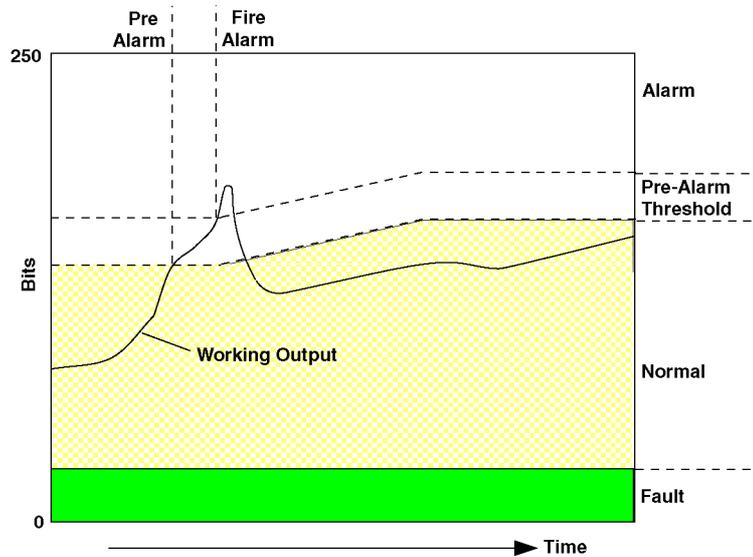
**Fig. 3 Pre-Alarm Threshold**
