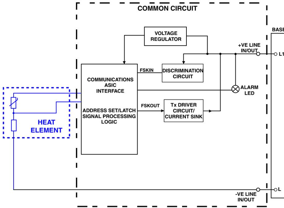
Fig. 1 Simplified Block Schematic Diagram
