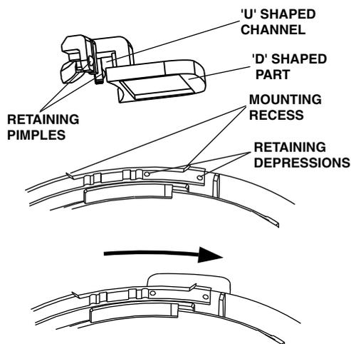
Fig. 5 Fitting Address Flag Carrier
