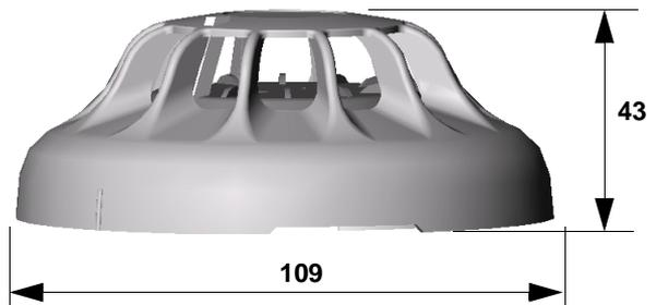
Fig. 3 Overall Dimensions of 801HEX detector
