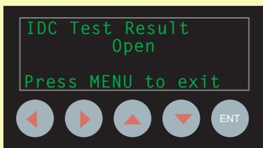
The screen is updated constantly, so the tester will display the state of the circuit (Normal, Open, Short) without any further menu commands. This makes it easy to test multiple IDC by moving the wires from one circuit to another.
