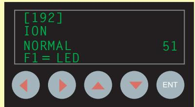
The display will show the lowest address of an abnormal device, and will indicate the fault.
