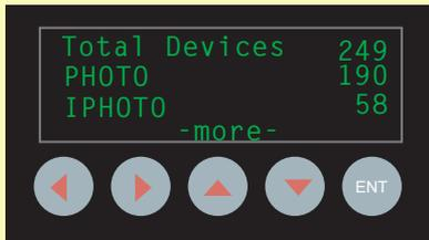
At the completion of the test, review the summary of devices detected. Then compare it to the devices that are supposed to be installed.
