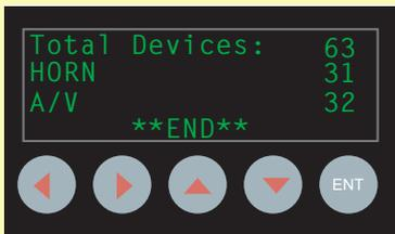
At the completion of the scan, review the summary of devices detected and compare to the list of devices that are supposed to be installed.
