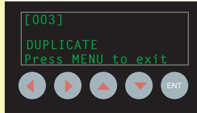
As with the IDNet devices, the TSIT sends the command to activate the device LED. In the example to the right, any device set to address 3 would have the LED ON. The installer can put the instrument down, but powered, and proceed to find the lighted LEDs to correct the address. Note that a missing address fault can often be explained by a duplicate device. It is useful to also take note of any missing devices before going out to correct duplicates.
