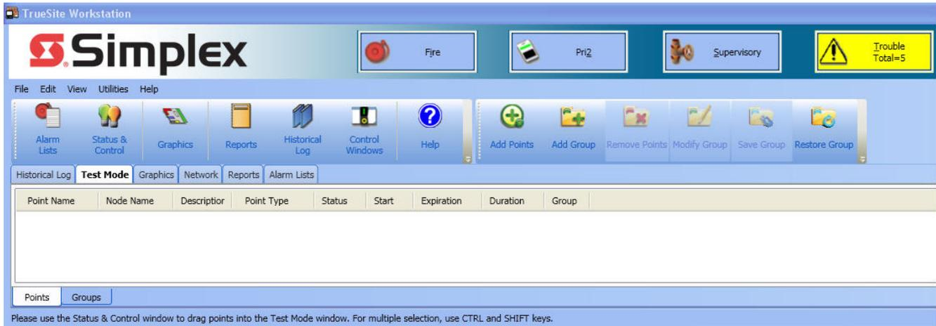
**Figure 7-19 Test Mode Tab with the Points Minor Tab Selected**
