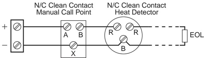
Legacy Thermal / Combined Circuit Wiring
