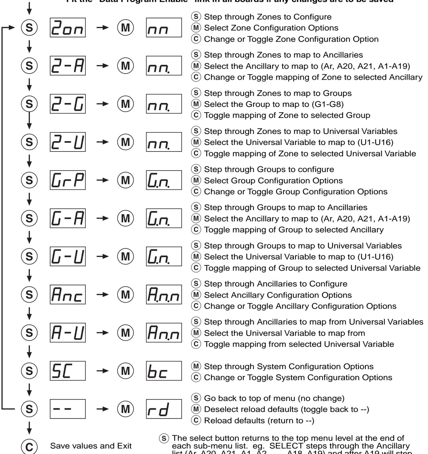
**(S)** The select button returns to the top menu level at the end of each sub-menu list. eg. SELECT steps through the Ancillary list (Ar, A20, A21, A1, A2 ... .. A18, A19) and after A19 will step back out to **Anc** and on to **A-U** etc. If, however, the SELECT button is pressed and held, it will continue to cycle through the sub-menu list until the button is released.
