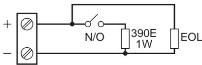
DBA/Evacuation Circuit Wiring
