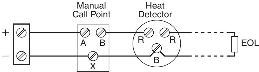
Thermal / Combined Circuit Wiring
