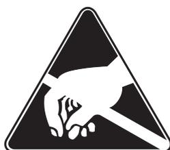
The FP1600 and OMEGA 64 Fire Alarm Systems contain Static sensitive components. Always observe appropriate ESD precautions when handling any Printed Circuit Boards.
