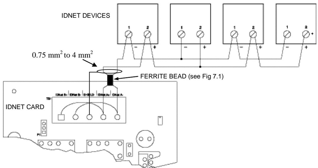
**Figure 7-4. Class B (spur or string) Wiring**
