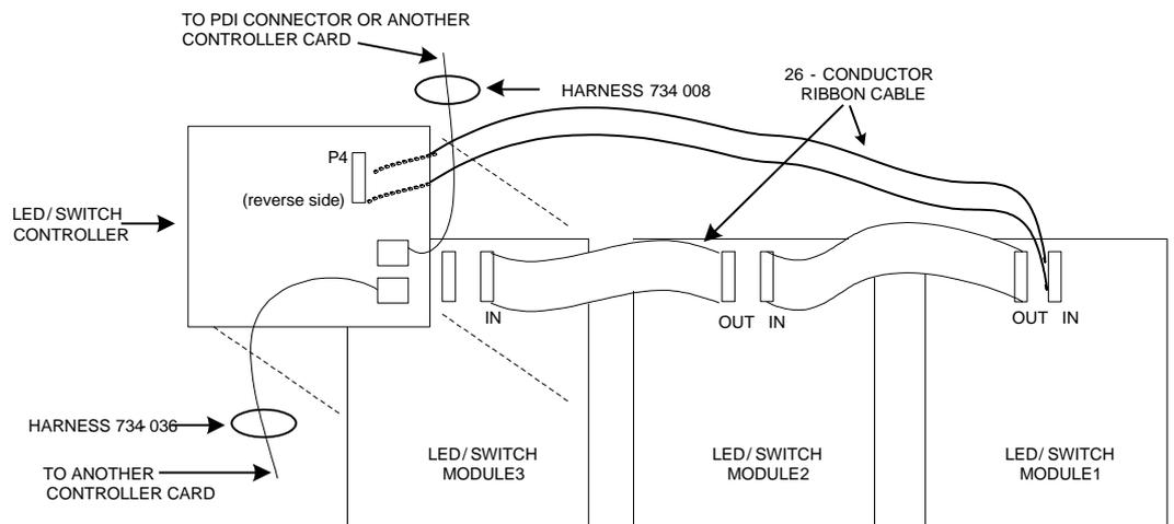
Figure 2-20. LED/Switch Controller Wiring
