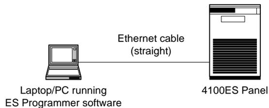
Figure 9-2. Ethernet Connection (fast)
