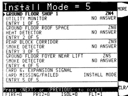
Figure 8-9. Displaying Contents of Install Mode List
