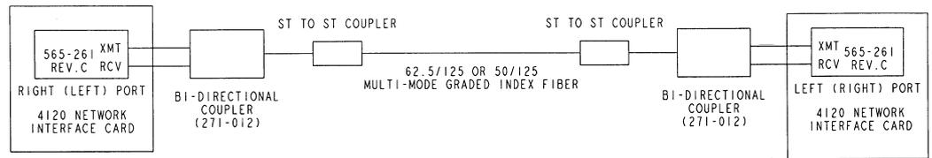
**Figure 4-7. Coupler Wiring**
