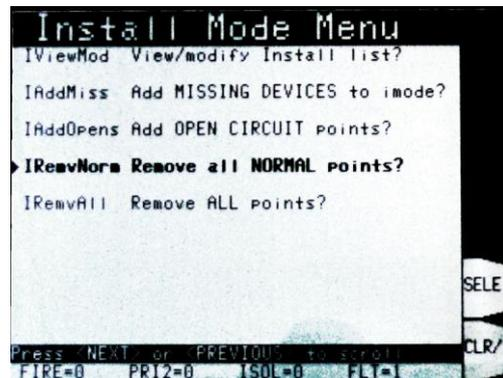
Figure 8-11. Remove Options on the Install Mode Menu Screen
