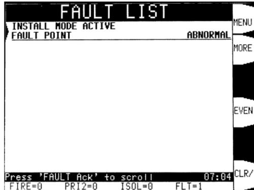
Figure 8-3. Fault List Now With Only a Single Install Mode Fault
