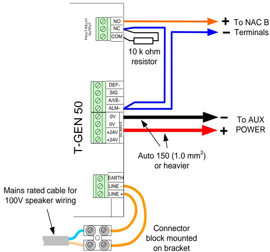
Figure 6-6. NAC Connection to a T-GEN 50
