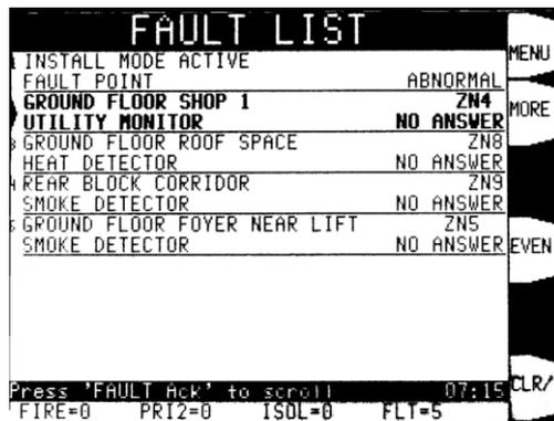
Figure 8-4. Fault List with Additional Missing Devices
