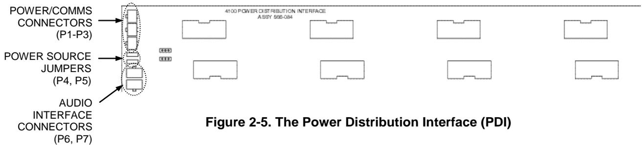
**Figure 2-5. The Power Distribution Interface (PDI)**
