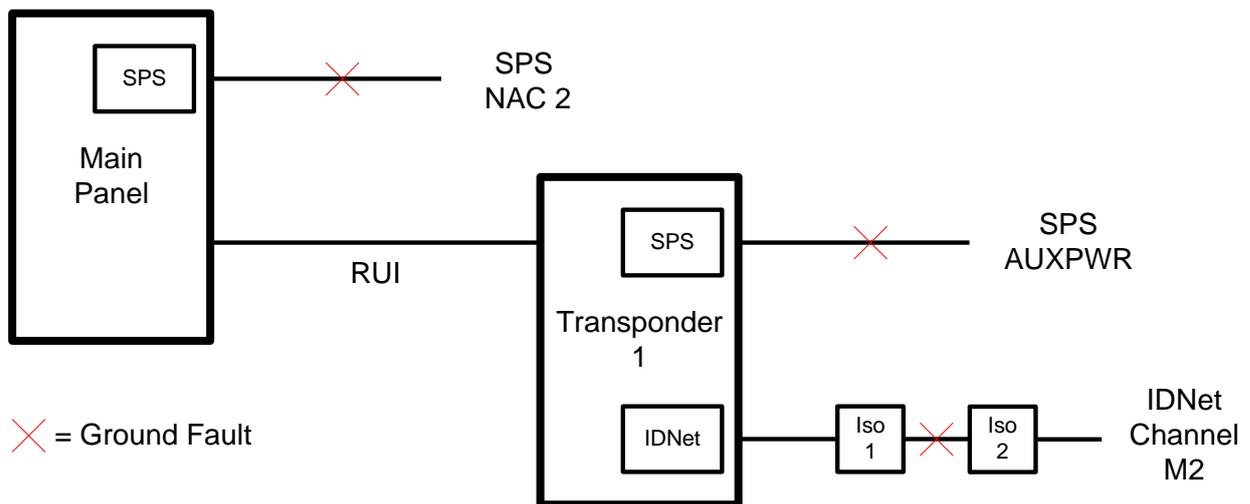
**Figure D-1. Earth Fault Example**
