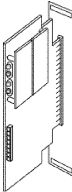
**Figure 4-5. Installing the NIC**
