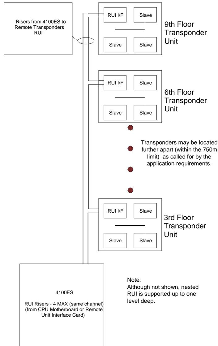
**Figure 1-2. MINIPLEX/RTU 4100ES System**
