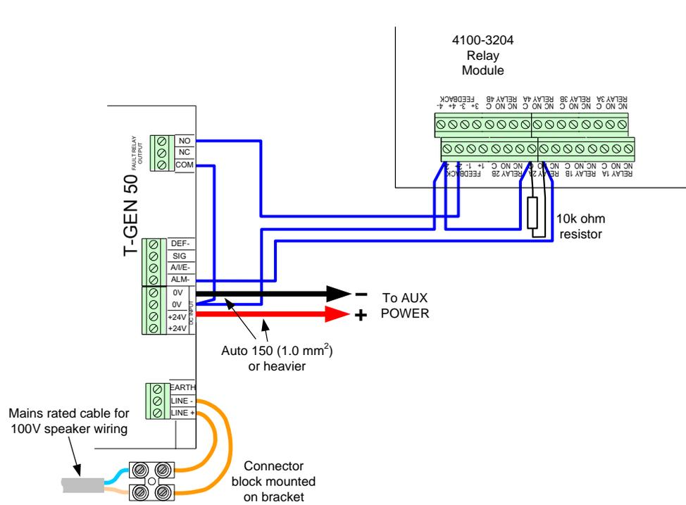
**Figure 6-5. Relay Module Connection to a T-GEN 50**
