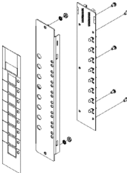
**Figure 2-19. Assembling / Disassembling the LED Display Card
