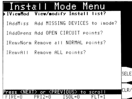
Figure 8-8. View Option on the Install Mode Menu Screen
