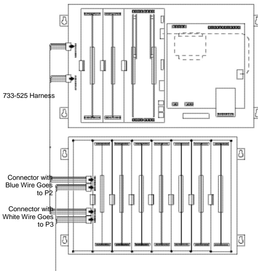
Figure 2-9. Power and Communication Wiring for Motherboards
