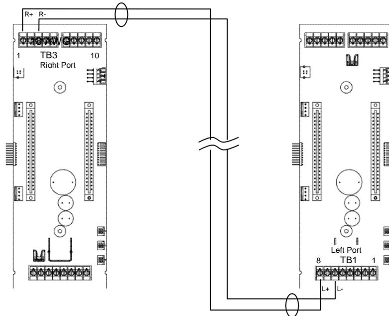
**Figure 4-8. Wired Media Interconnections between 4100ES Master Motherboards**
