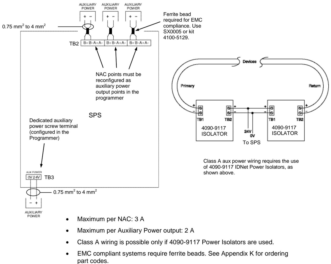
**Figure 6-8. Auxiliary Power Wiring**
