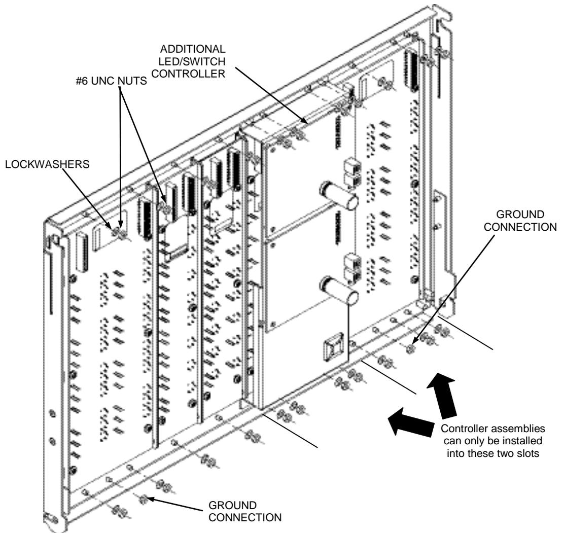
**Figure 2-17. LED/Switch Card Mounting on a bay mounted door
