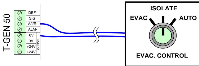
**Figure 6-7. Wiring an Evacuation Controller to a T-GEN 50**
