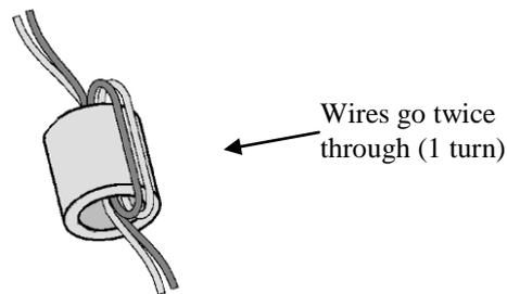
**Figure 6-1. The Ferrite Bead**
