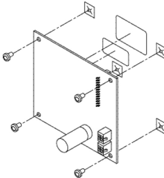
**Figure 2-18. Controller Card Mounting**
