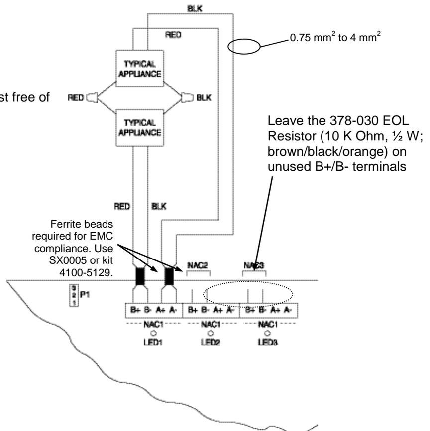
Figure 6-2. Class A NAC Wiring
