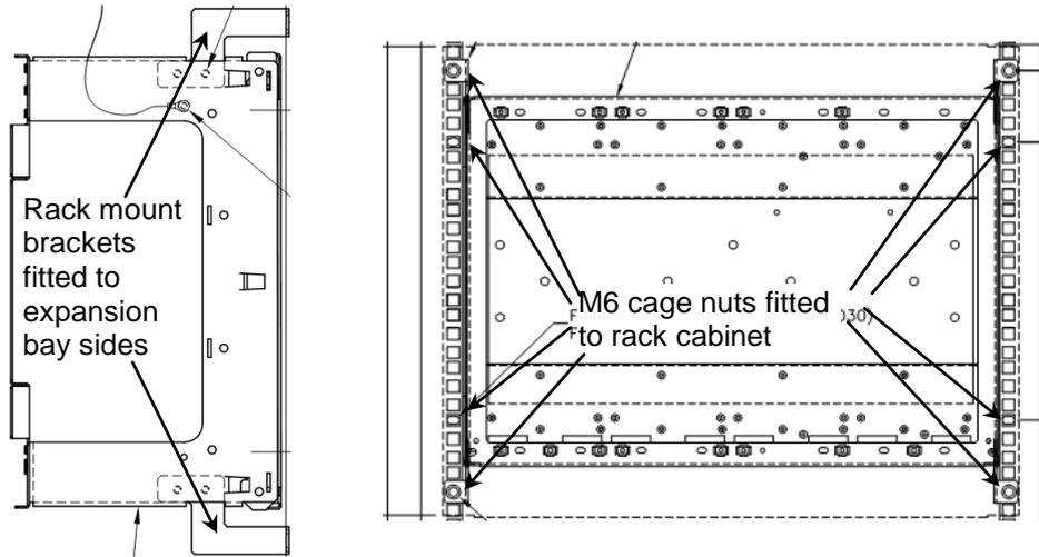
**Figure 2-6. Bracket and Bay Mounting – earlier style**
