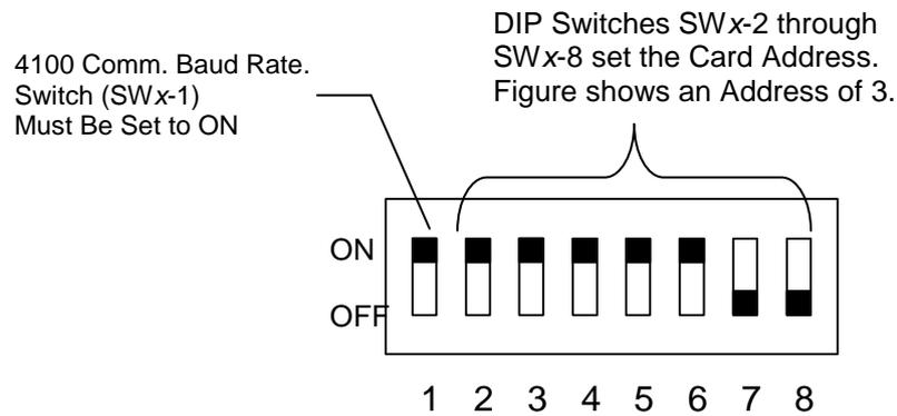
Figure A-1. DIP Switch SW<sub>x</sub>
