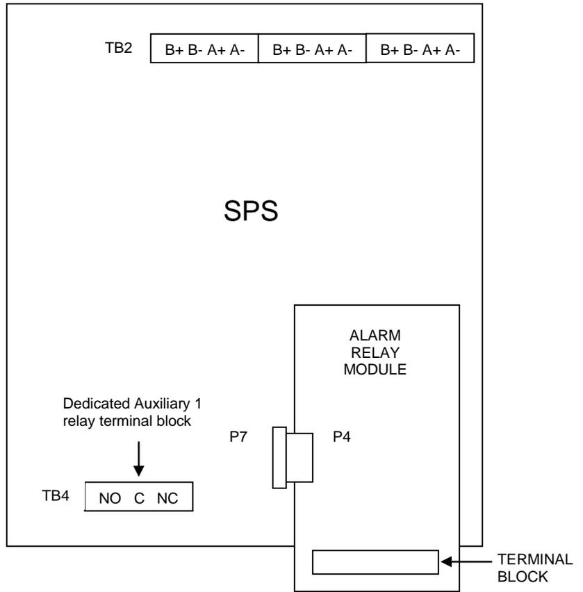
**Figure 6-9. Auxiliary Relay & Alarm Relay Card Relays**
