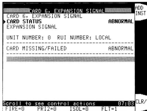
Figure 8-2. Moreinfo on this Fault with Add Inst Option
