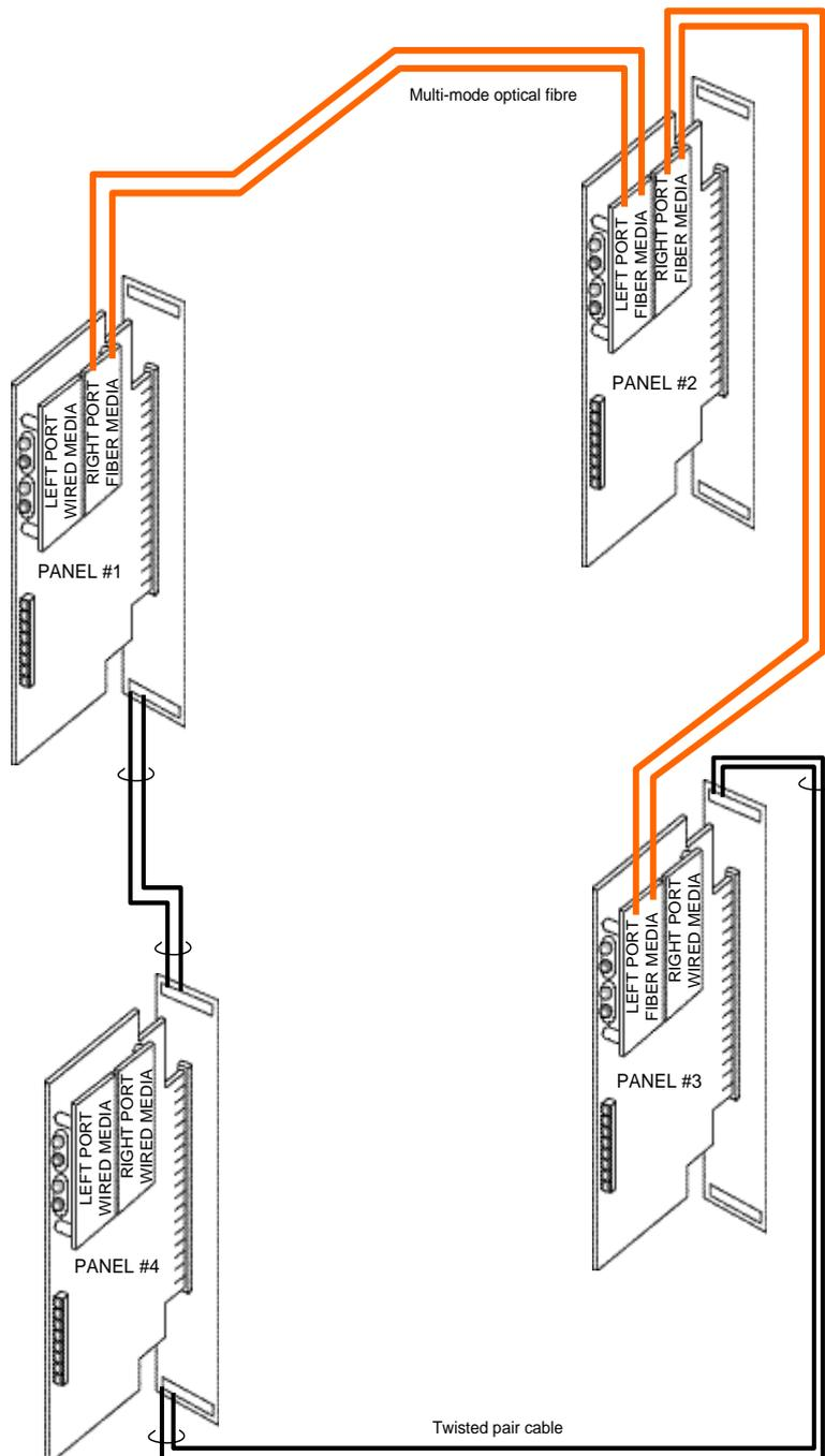
Figure 4-9. Example of Ring/Loop Network Wiring
