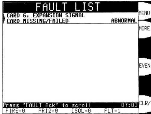
Figure 8-1. Sample Fault List Display Showing a Missing Card
