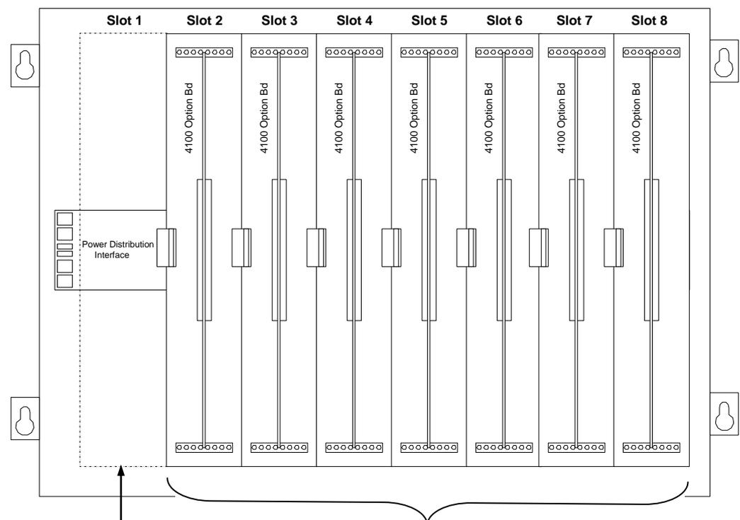
This slot cannot contain a motherboard unless the pins on P1 (or leftmost pin connector) are removed.
