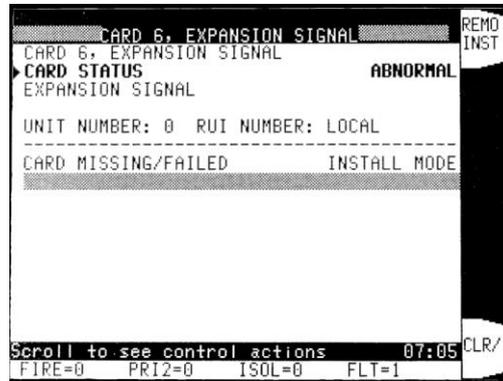
Figure 8-10. More Info on a Device in the Install Mode List
