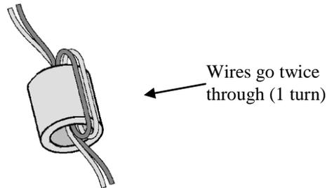
**Figure 7-1. Ferrite Bead Wiring**
