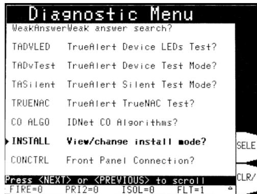
Figure 8-6. Install Mode Option on Diagnostic Menu Screen
