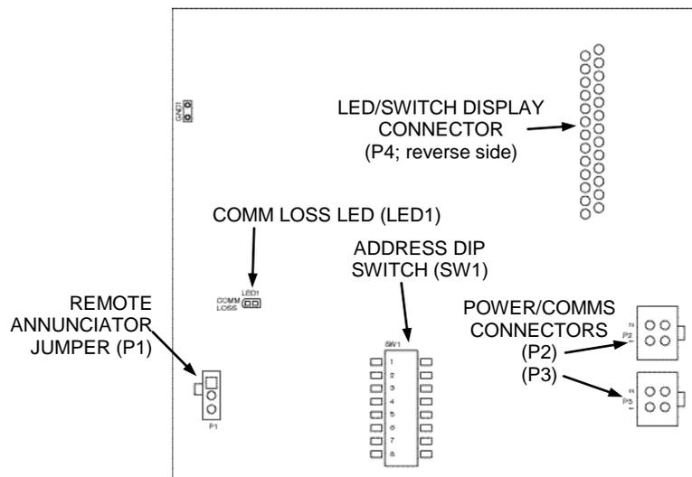
**Figure 2-16. LED/Switch Controller**
