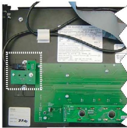
**Figure 3 – Correct orientation of the Ethernet download card on a 2x40 LCD door**
