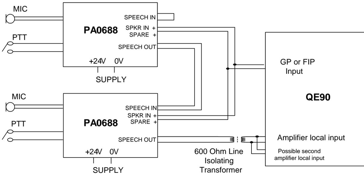
**Figure 2 - Using PA0688 Pre-amp with QE90 Local Inputs**
