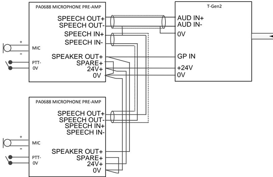
Figure 4 – Microphone Pre-Amp to T-Gen2
