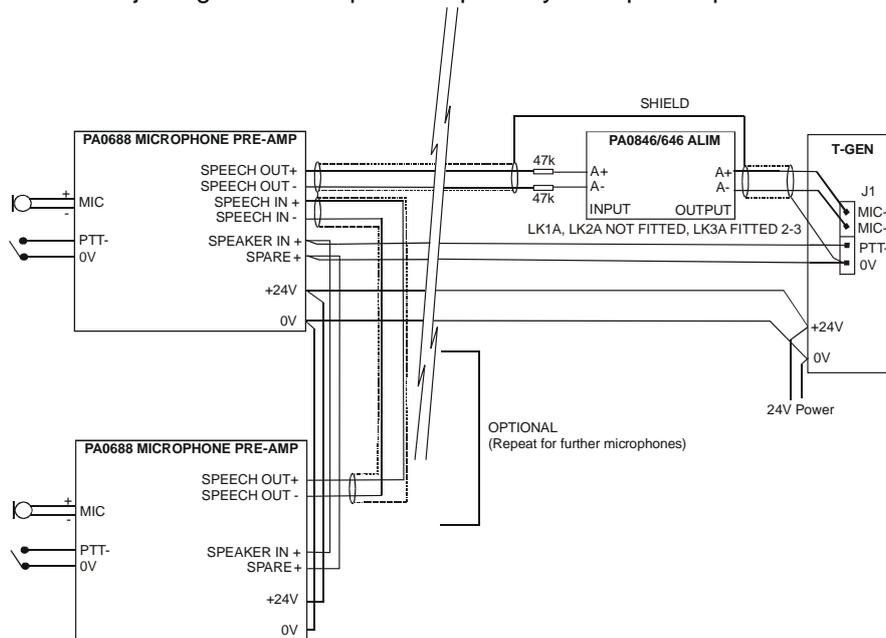
**Figure 7 - Remote Emergency Microphone(s) for T-GEN 50**
