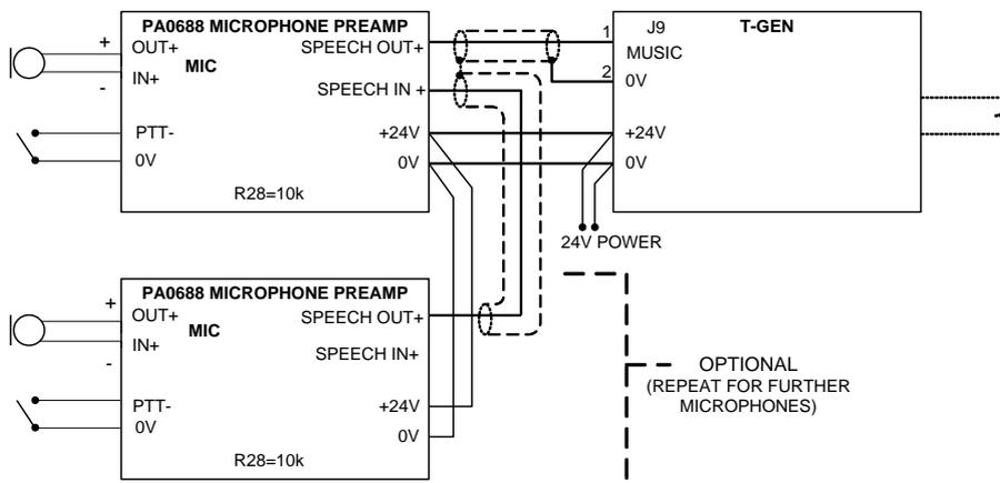
Figure 5 - Unbalanced Configuration, PA0688 to T-GEN 50, Non-emergency Microphone
