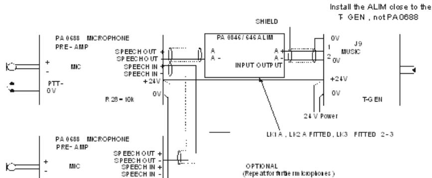
**Figure 6 - Balanced Configuration, PA0688 to T-GEN 50, Non-emergency Microphone**
