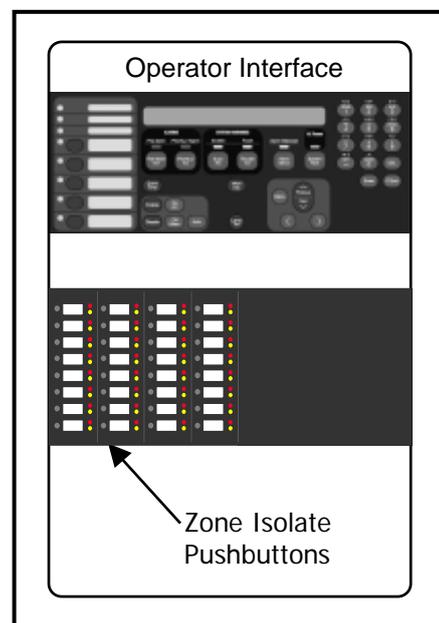
*The panel is reset by pressing SYSTEM RESET. If the alarm won't reset the point may still be activated. Press FIRE ALARM ACK when the point alarm is displayed, then press DISABLE, ENTER. Press FAULT ACK (to acknowledge the fault caused by disabling a point), then press SYSTEM RESET again. The disabled detector must be re-enabled when the condition is cleared.*
