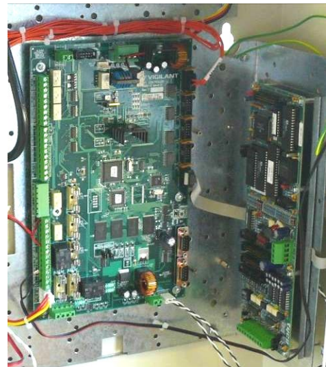
Figure 14.3 – I-HUB Mounted on 15U Gearplate RHS Flange
