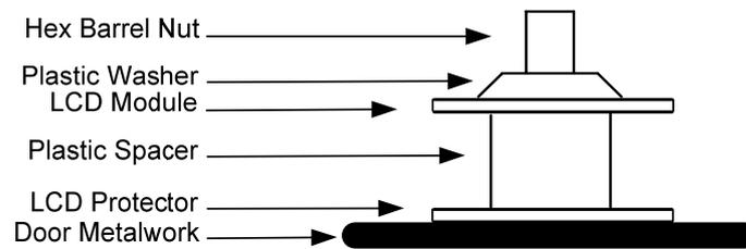
**Fig. 1 – LCD Module Mounting – Ensure Plastic Washers Fitted**
