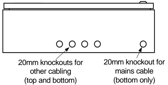
Figure 3 – Knockout positions on Slimline cabinet
