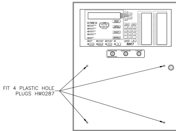
Figure 8 - Positions of Push-in Fasteners HW0287
