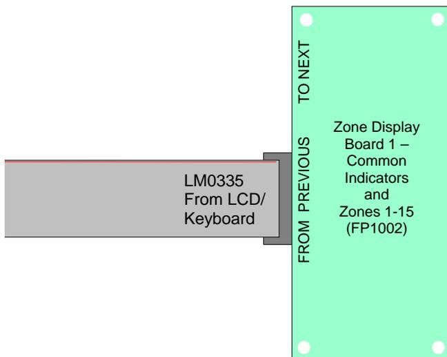
Figure 4 – Single Zone Display on gear plate (Rear Service format)
