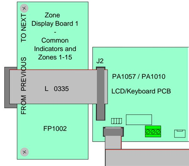
Figure 6 – Single Zone Display on front panel (Front Service format)
