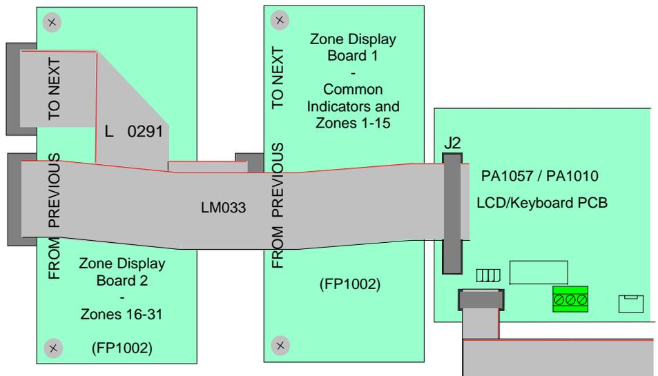
Figure 7 – Double Zone Displays on front panel (Front Service format)
