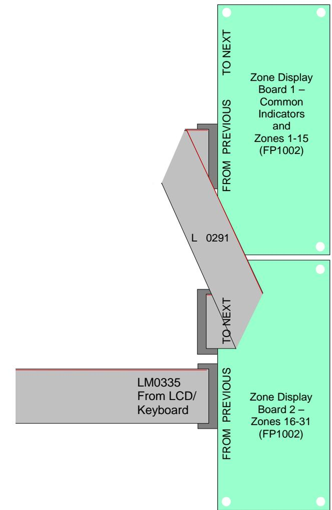
Figure 5 – Double Zone Displays on gear plate (Rear Service format)
