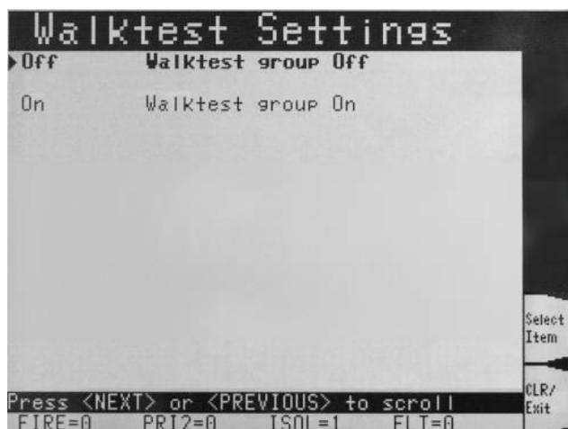
In the settings display, the highlight shows the current setting. Use Up or Down to move the highlight to the other setting, then <Select Item> soft key to change it.
