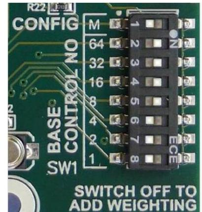
Figure 10 – DIP Switch Setting (Master and base control no = 7)
