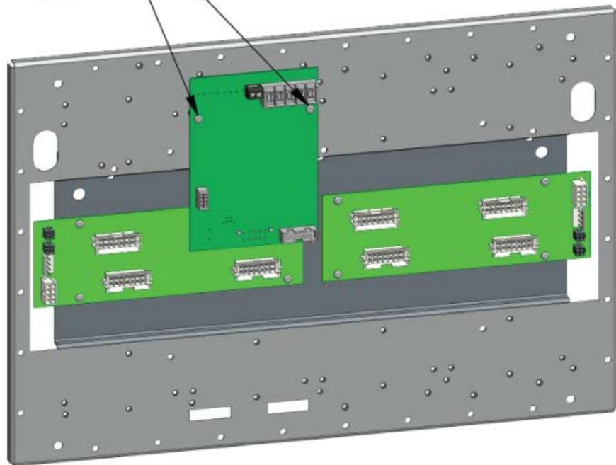
In the 15U RTU, there is space for three additional PDI cards on the backplane.
