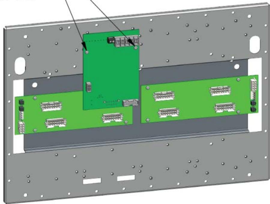
Plug the card into the socket on the backplane, and secure it with the two screws supplied with the card. The card draws power and communications from the PDI backplane. For information about field wiring, refer to *LT0432 Field Wiring Diagrams*.
