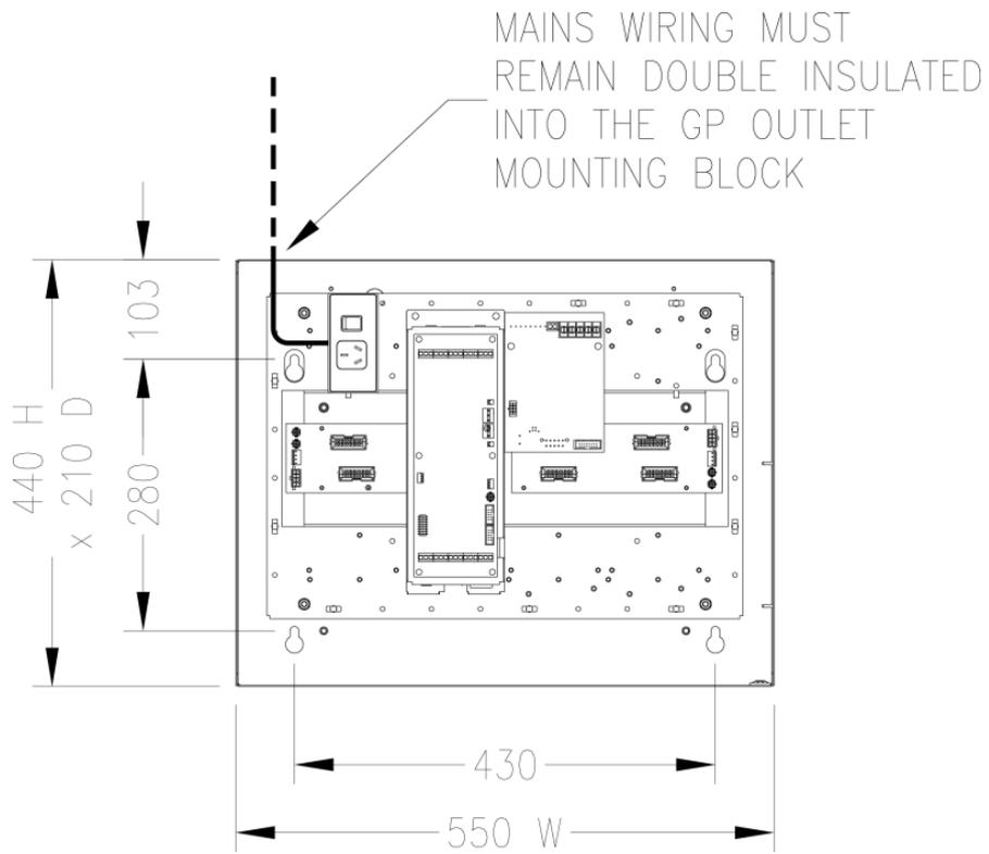
Figure 59. Mounting a 15U cabinet RTU
