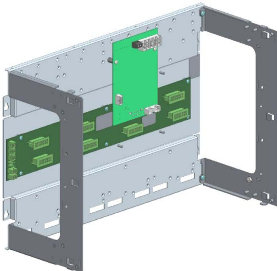
Plug the card into the socket on the backplane, and secure it with two screws supplied with the card. For information about field wiring, refer to the appropriate drawings in *LT0432 4100ESi Field Wiring Diagrams*. Information about using the 4100-5013 8 Zone/Relay Card are in [Chapter 7](#).
