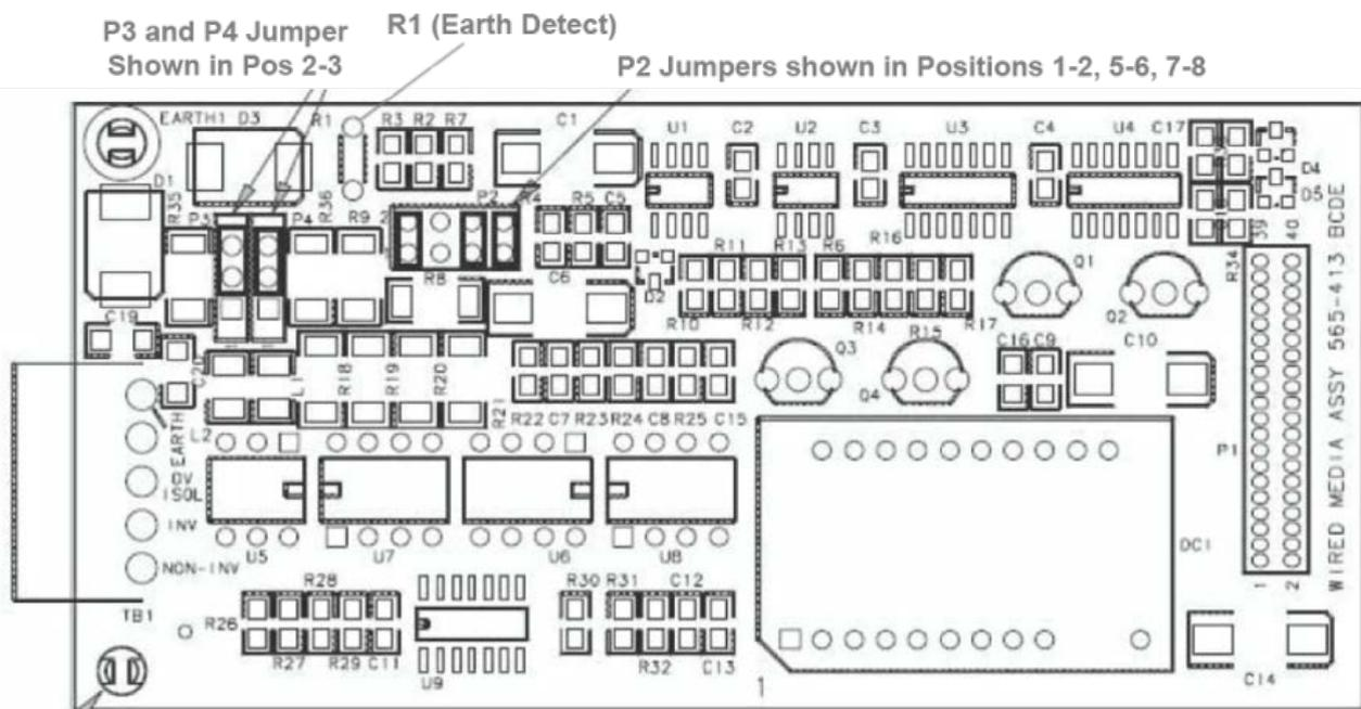
**P2:** Selects the wire type. Fit positions 1–2, 5–6, and 7–8 for 1.0 mm<sup>2</sup> or heavier paired wiring. Remove all jumpers for twisted pair telephone cable wiring.
