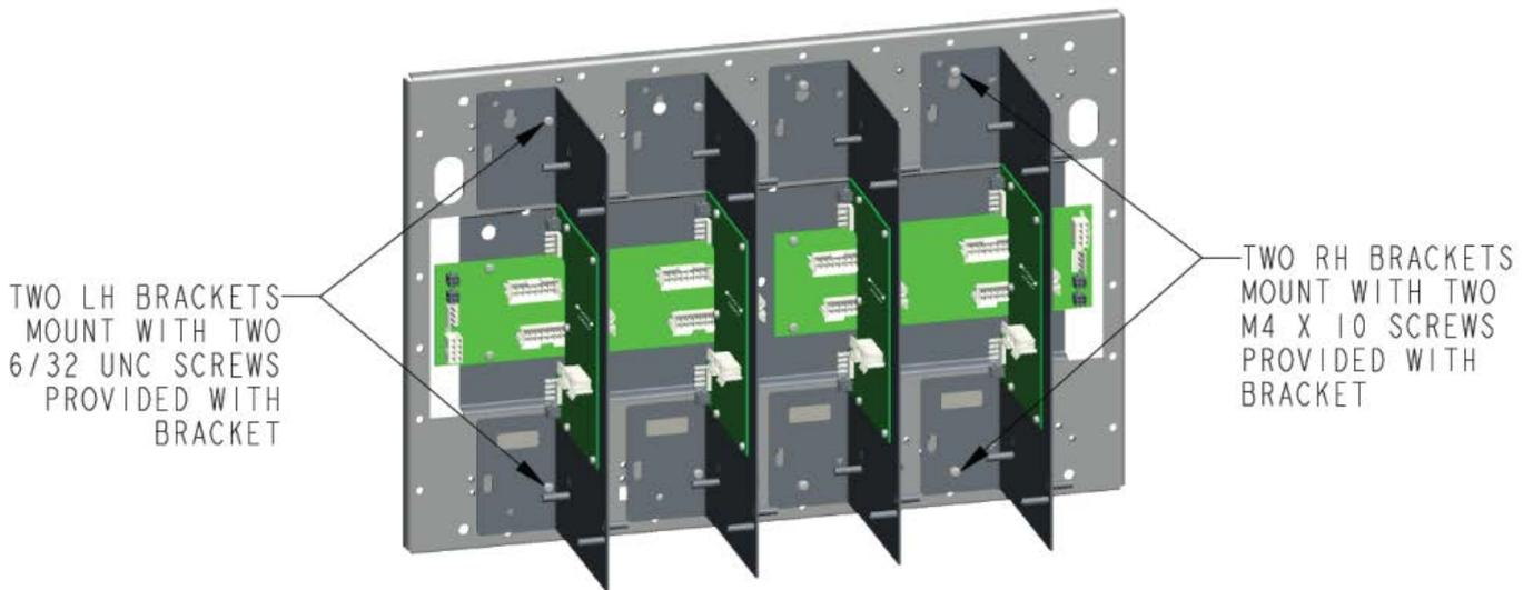
There are four possible mounting positions for the ME0516 in an 8U expansion cabinet. The recommended mounting position for the 4 100-6072/6073 SM Fibre Modem is at the left. See [Figure 34](#).
