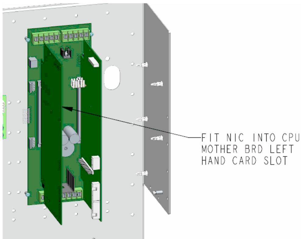
Before fitting the NIC, set the jumper settings on the NIC, the CPU motherboard, and the media cards correctly. Refer to *LTO6 15 Media Card Installation Instructions* for details on mounting the media cards on the NIC, and then install the NIC on the CPU motherboard.
