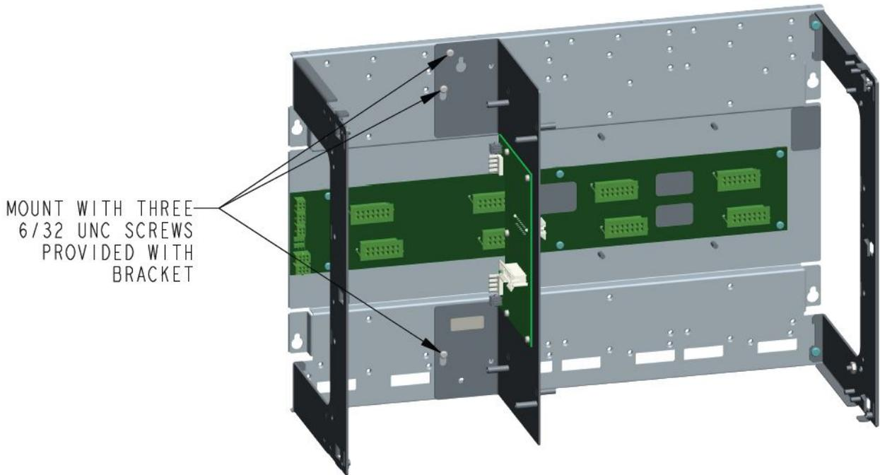
Expansion bay mounting in four possible positions. The recommended expansion bay mounting for 4100-6072/6073 SM Fibre Modems is at the left to avoid colliding with other cards due to the overhang. See Figure 34.
