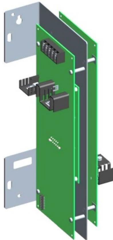
Figure 29. Mounting two 4100-6072/6073 SM fibre modems
