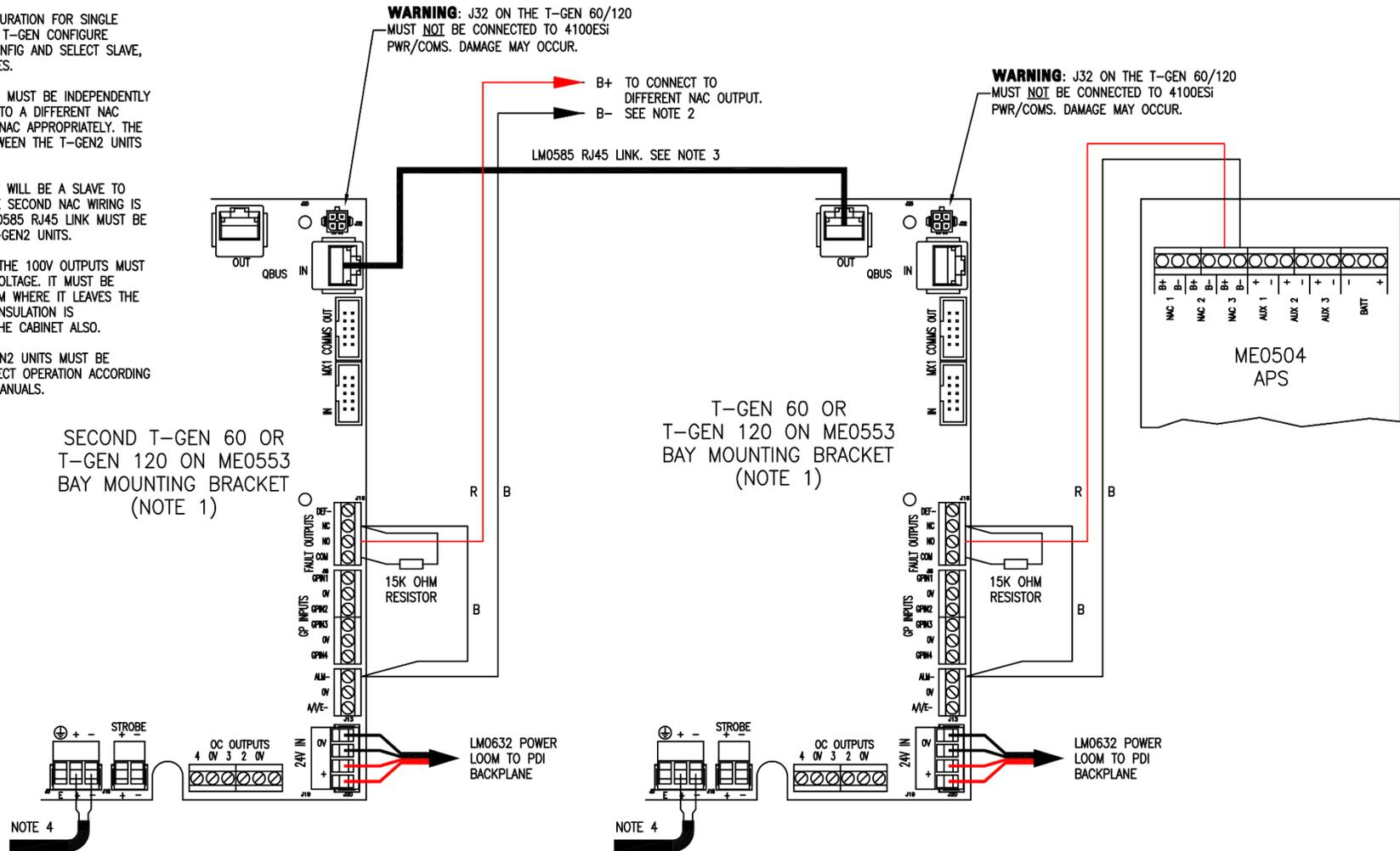
Figure 46. Wiring for T-GEN 60 and T-GEN 120 with switching modules
