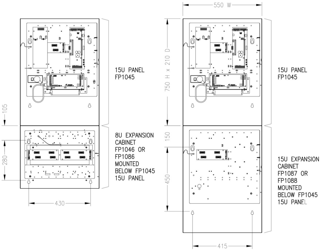
Figure 19. Mounting cabinets side by side
