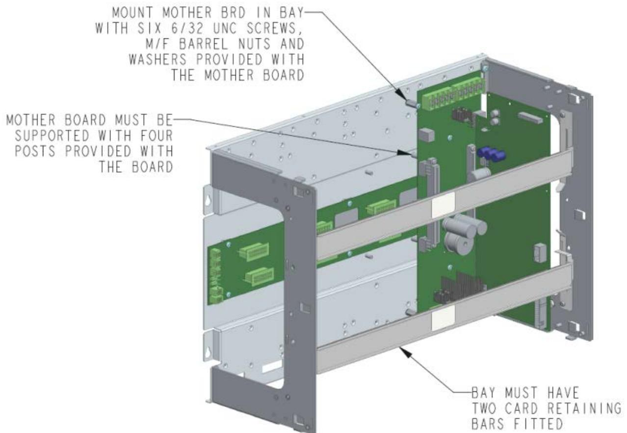
Legacy cards require bars to hold them in place. You can use a pair of retaining bars as shown in Figure 40, or a single central retaining bar (ME0565). The central bar is required when legacy cards and an APS power supply are located in the same bay. The retaining bars are supplied with the bays in BTO systems.
