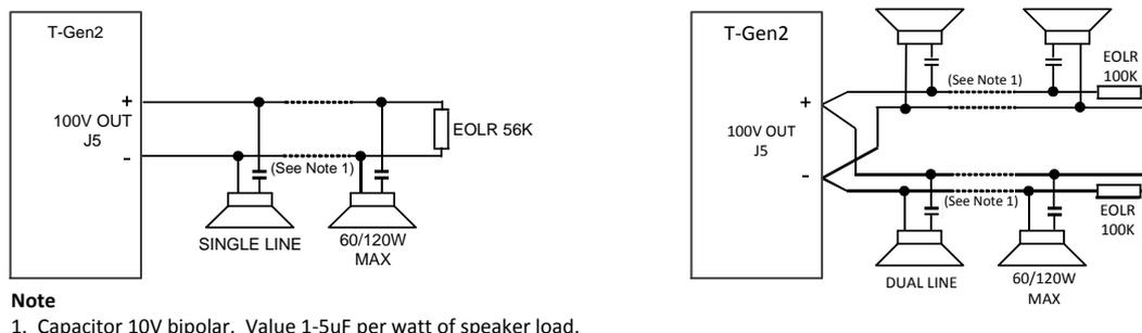
Figure 2.1 100V Speaker Line Wiring
