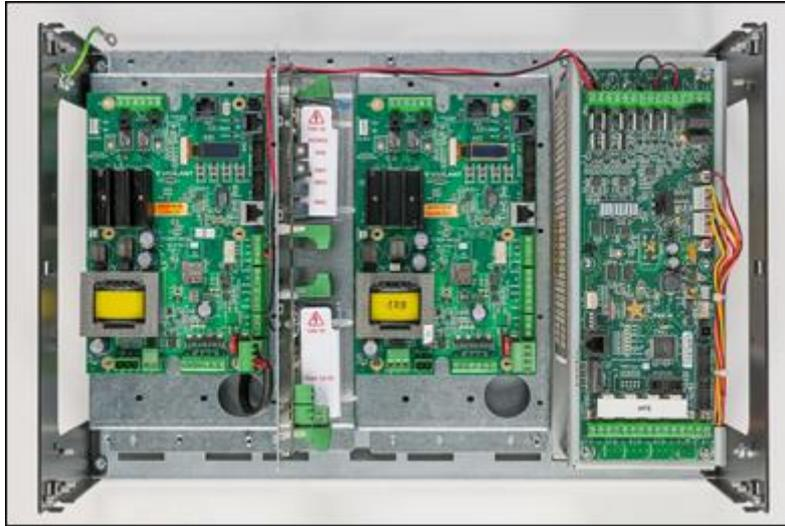
Fig 1.B Mounting T-Gen2 in 4100ESi with APS and 100V Modules
