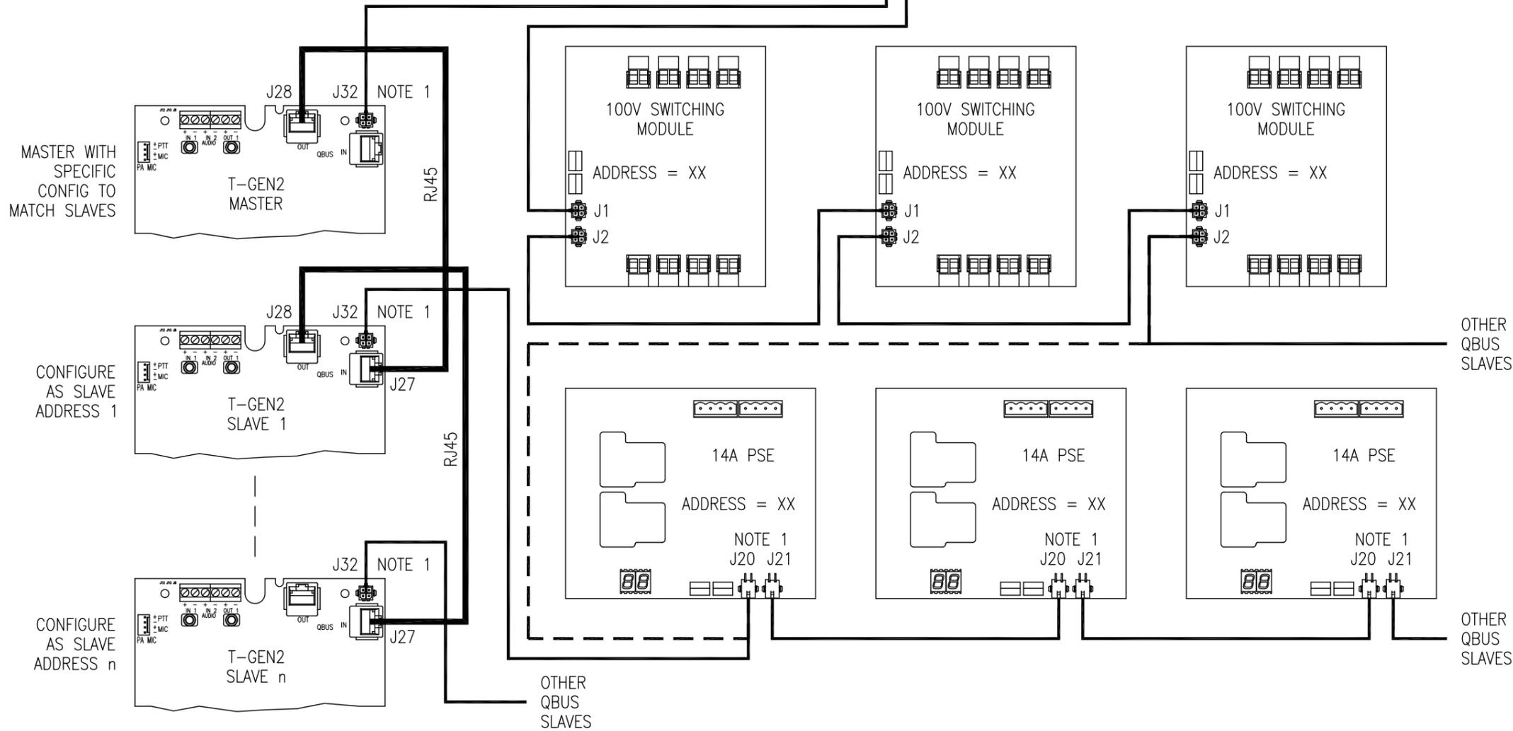
QBUS IS A DAISY-CHAIN/STAR COMMS BUS FROM THE MASTER T-GEN2 TO EACH OF THE SLAVE QBUS DEVICES.
