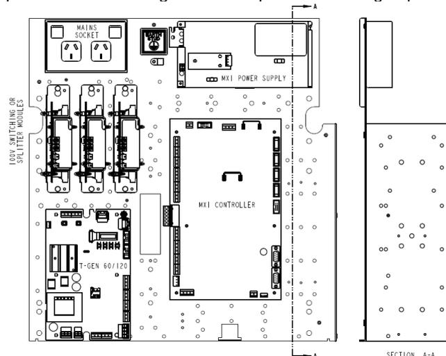
Fig 1.A Mounting T-Gen2 on MX1 gearplate
