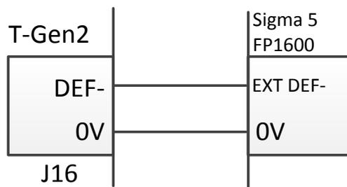
Figure 3.8 DEF- Connection to NZ Panels
