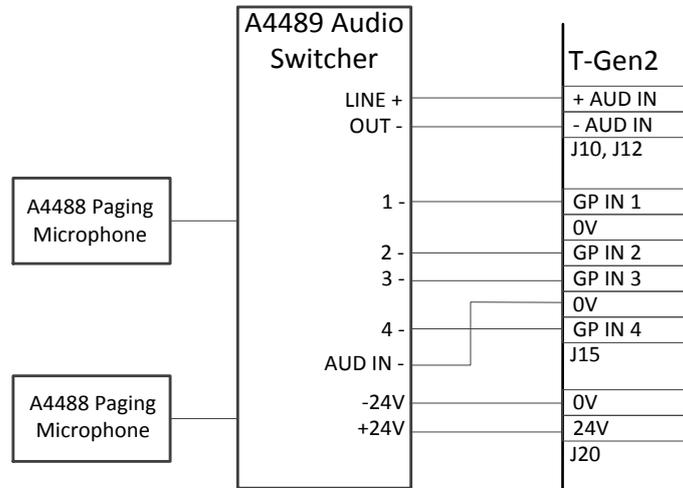
Fig 3.15 4-Area Paging Console Connections
