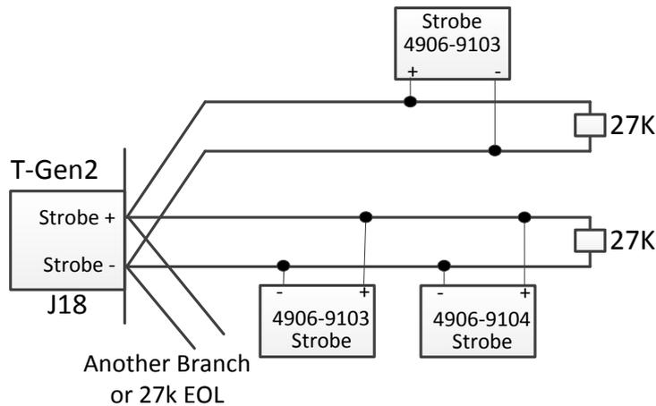
Fig 3.7 Strobe Wiring
