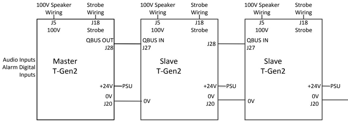
Figure 3.10 Slave T-Gen2 Wiring
