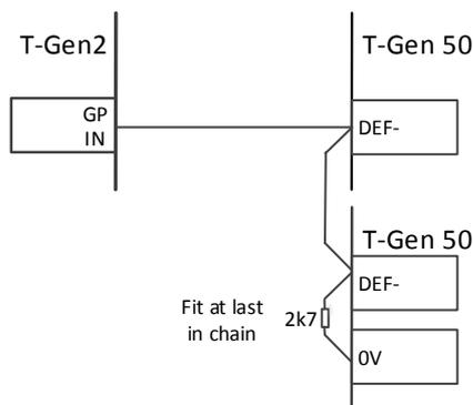
Figure 3.11B Fault Supervision Using DEF- Outputs
