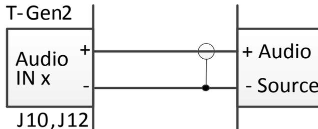
Fig 3.4 Audio Input Connections
