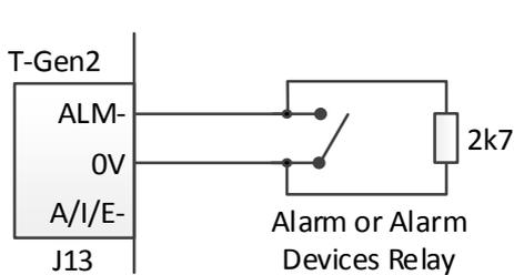
Fig 3.3A Fire Alarm Input Wiring (Supervised)
