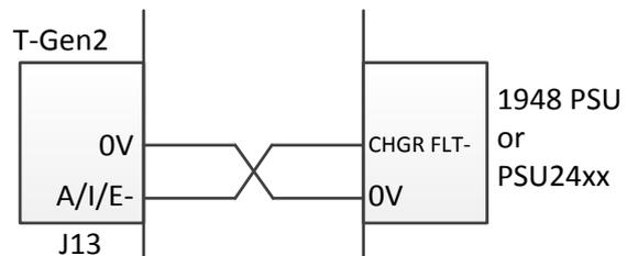
Fig 3.3D AIE Input Used For External PSU Fault
