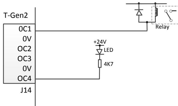
Figure 3.9 Example Open Collector Wiring
