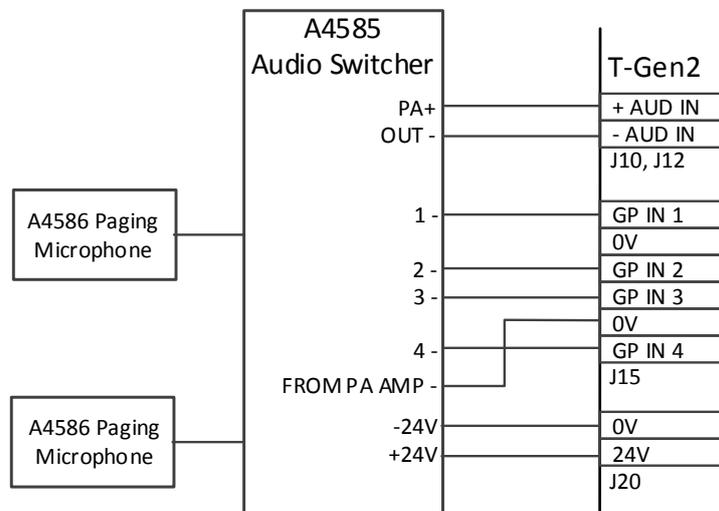
Fig 3-16 16-Area Paging Console Connections
