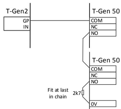
Figure 3.11C Fault Supervision Using T-Gen 50 Fault Relays
