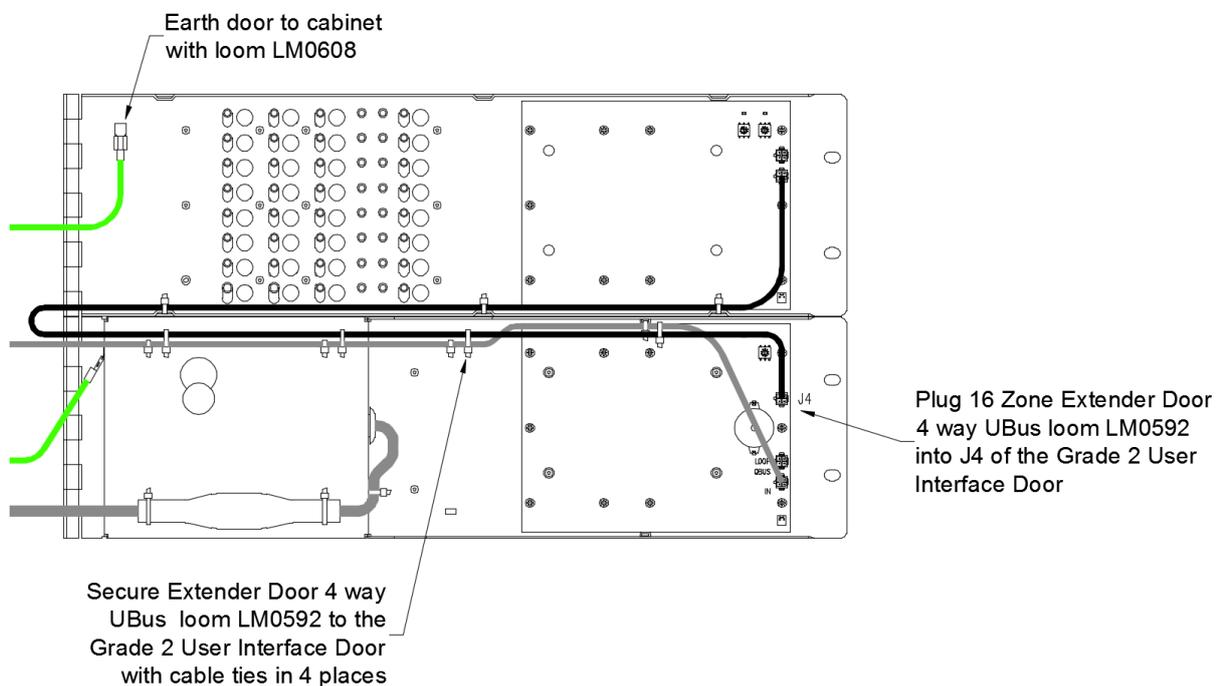
Figure 3 – Grade 2 16 Zone Extender Door Wiring
